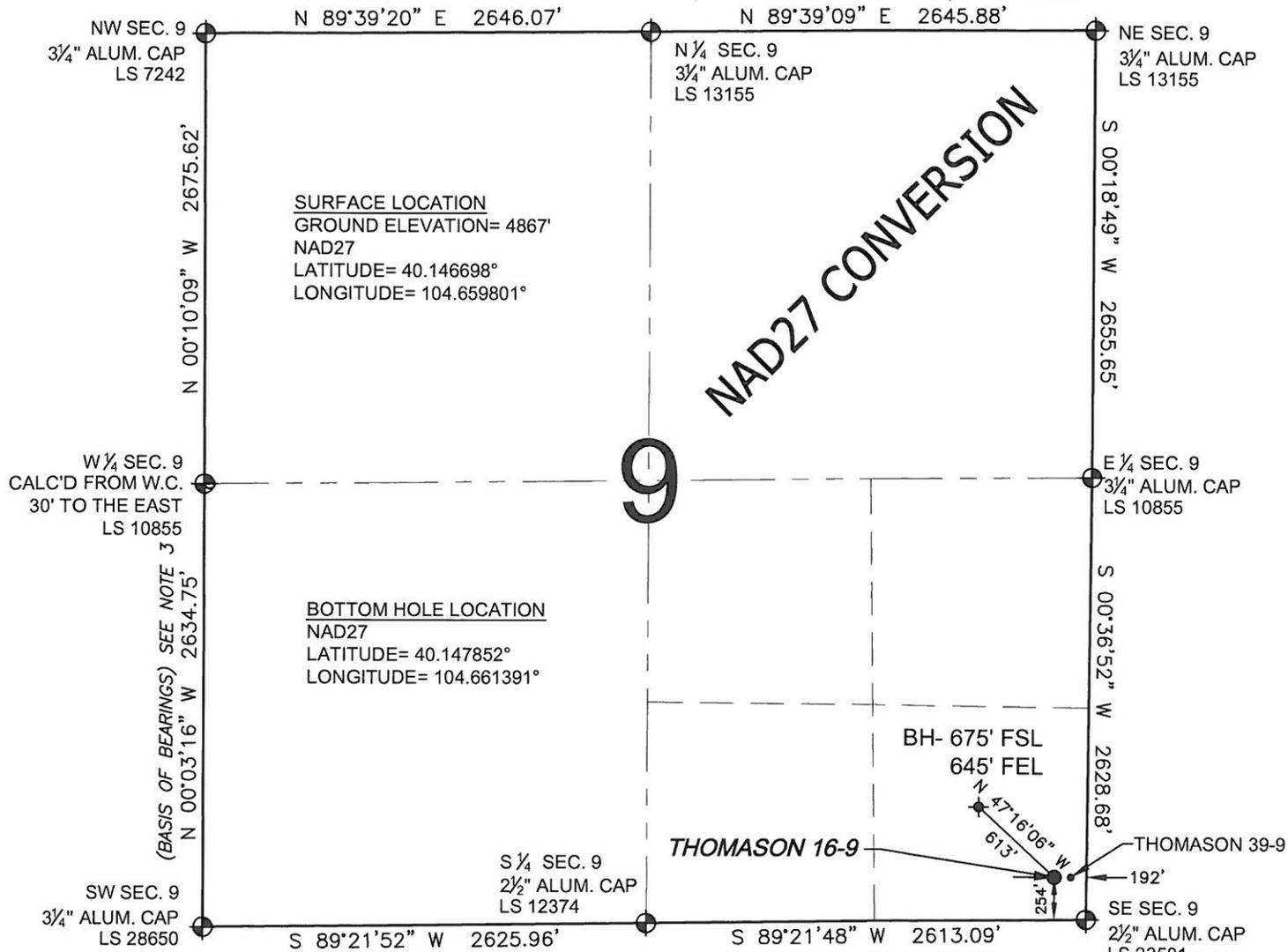
WELL THOMASON 16-9 TO BE LOCATED 254' FSL AND 192' FEL, SECTION 9, T2N, R65W OF THE 6TH P.M.
