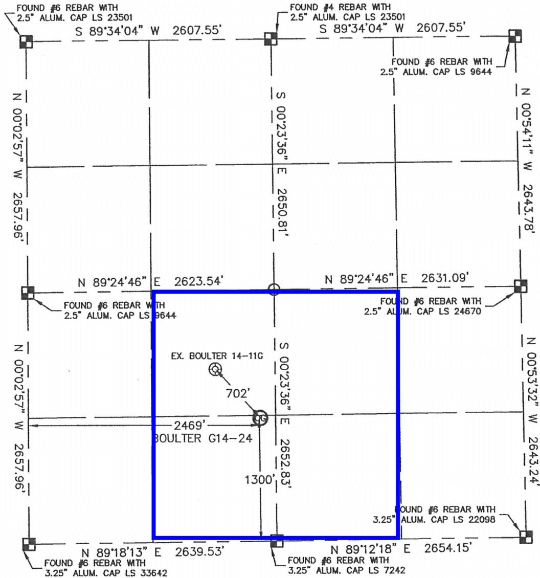
In accordance with a request from Mike Rodine with Noble Energy Inc. Lat40°, LLC has determined the surface location of the BOULTER G14-24 to be 1300' from the SOUTH line and 2469' from the WEST line as measured at right angles from the section line of Section 14, Township 4 North, Range 65 West of the Sixth Principal Meridian, County of Weld, State of Colorado.
