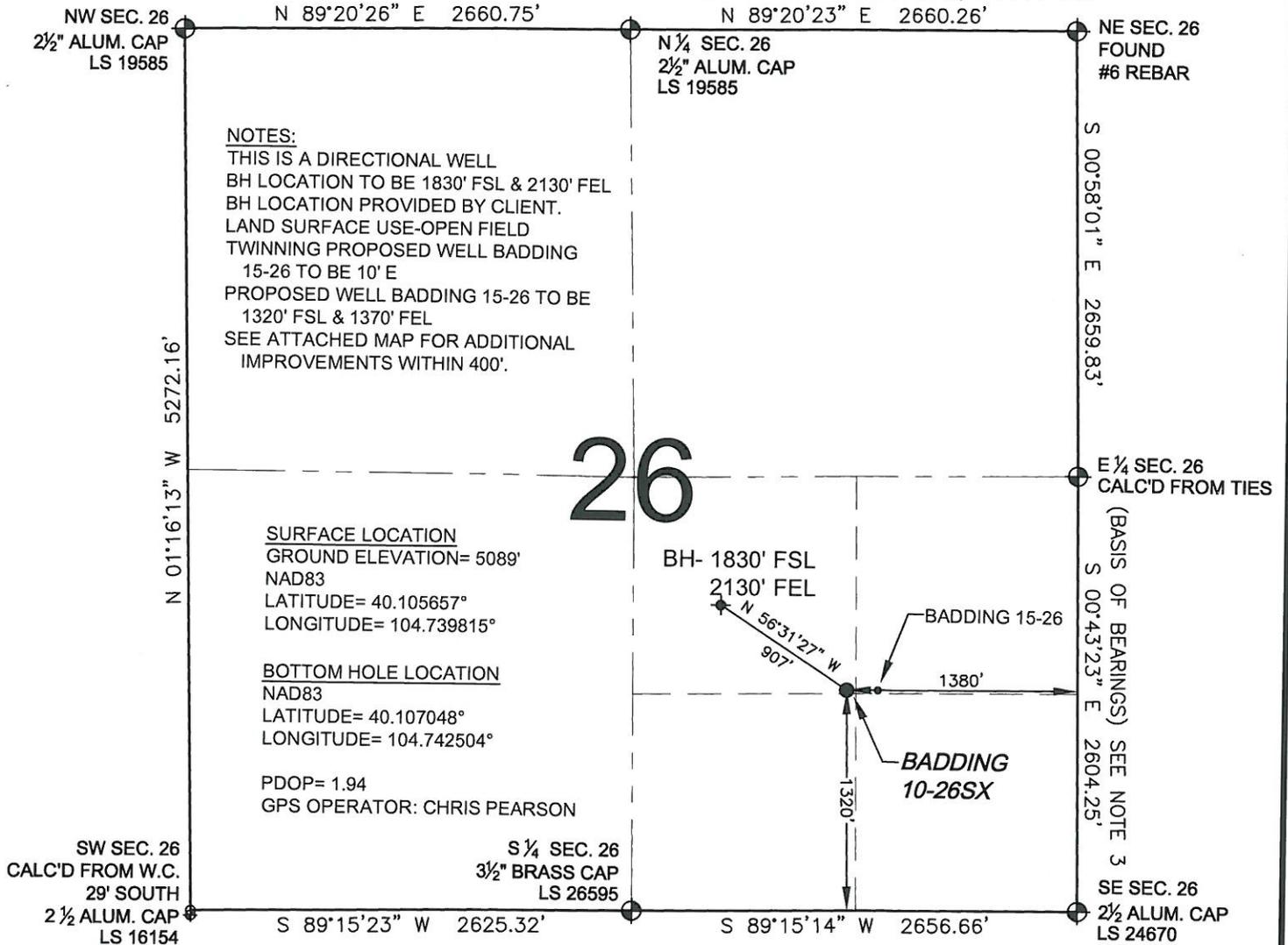
WELL BADDING 10-26SX TO BE LOCATED 1320' FSL AND 1380' FEL, SECTION 26, T2N, R66W OF THE 6th P.M.
