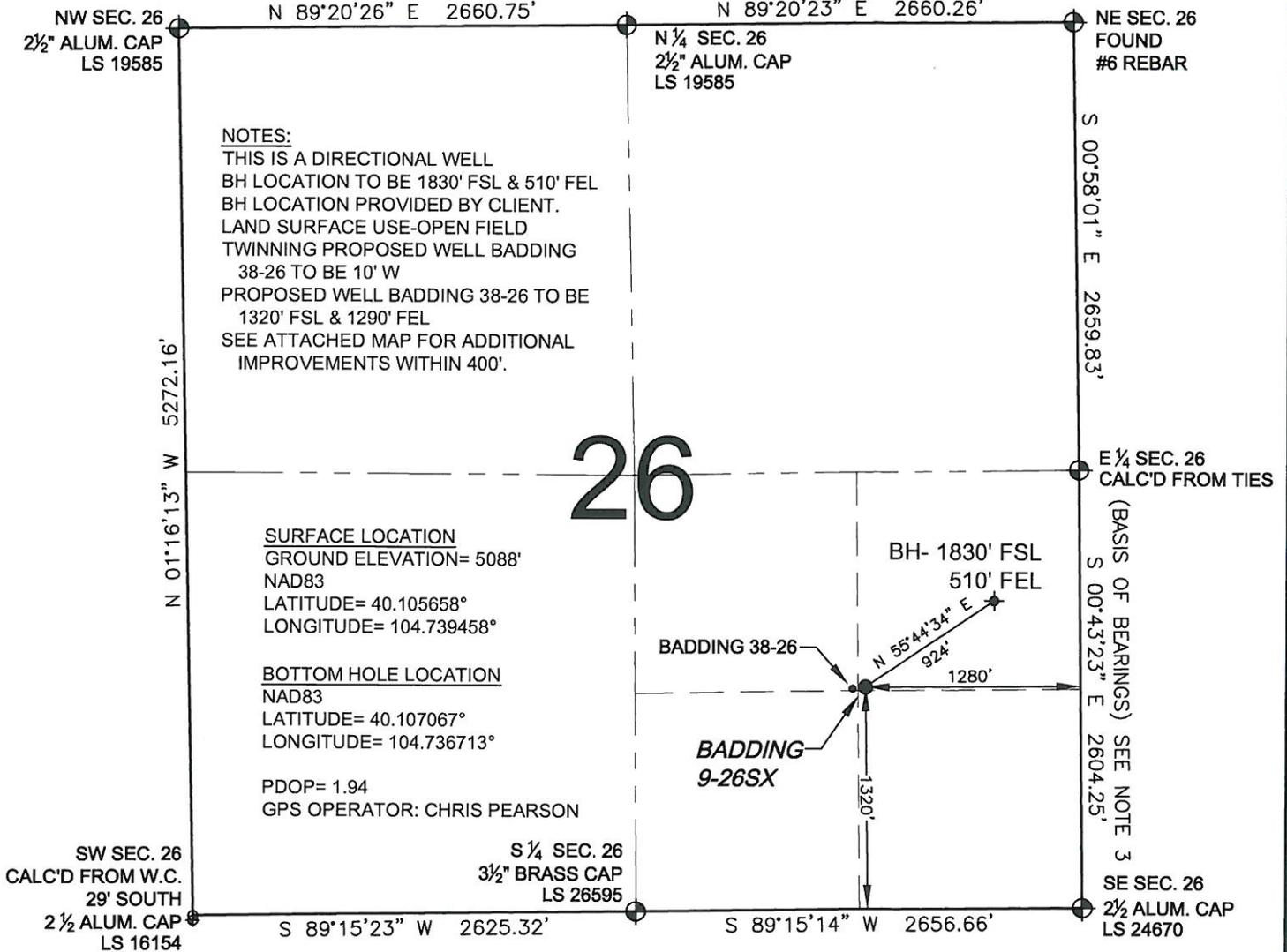
WELL **BADDING 9-26SX** TO BE LOCATED 1320' FSL AND 1280' FEL, SECTION 26, T2N, R66W OF THE 6th P.M.
