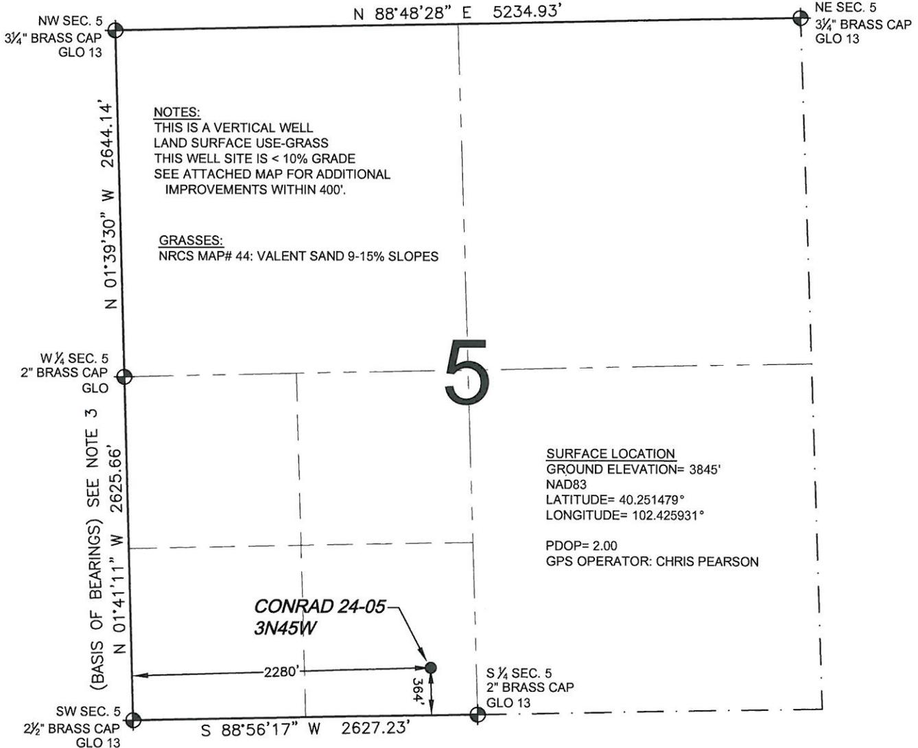
WELL **CONRAD 24-05 3N45W** TO BE LOCATED 364' FSL AND 2280' FWL, SECTION 5, T3N, R45W OF THE 6th P.M.
