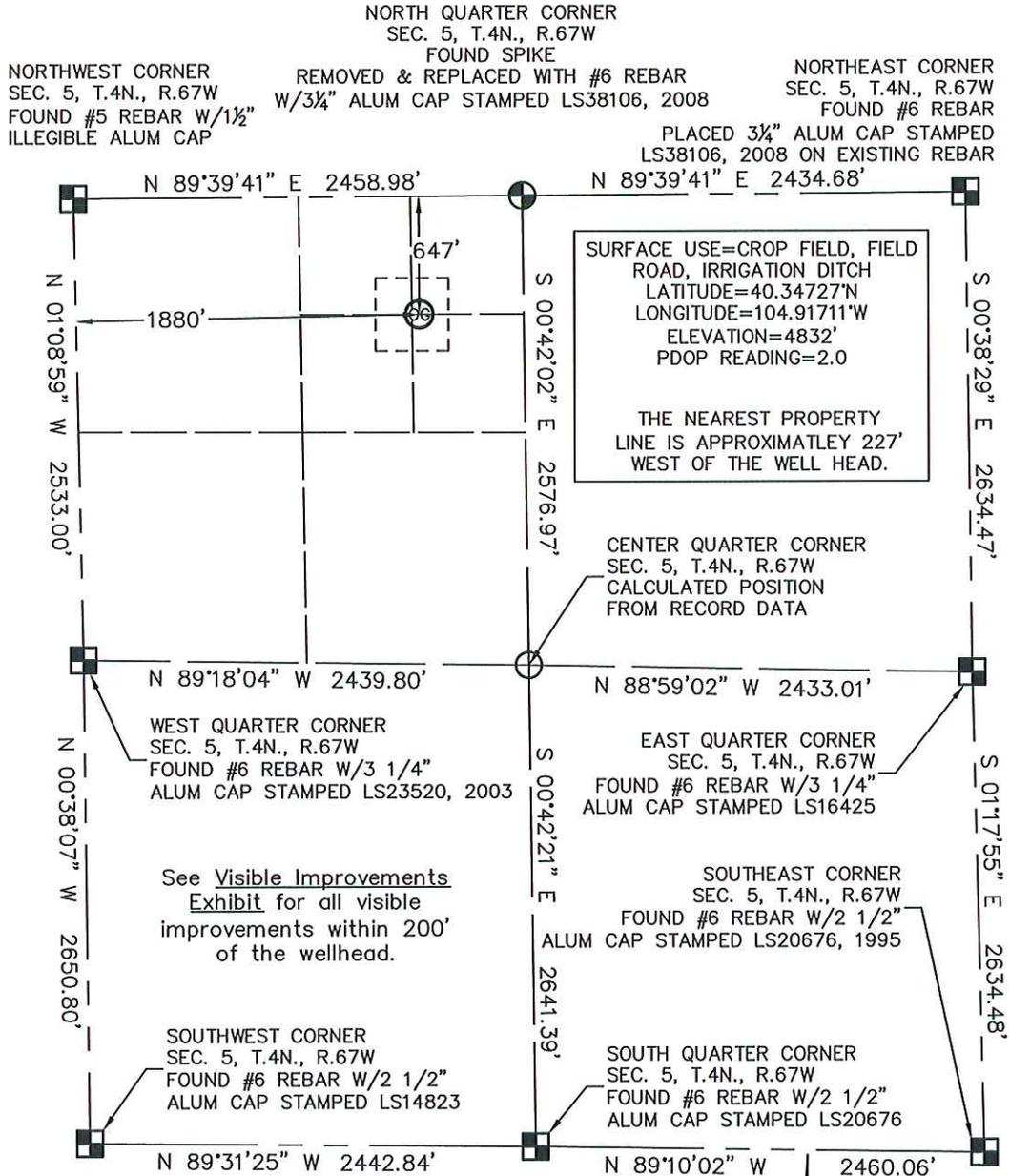
King Surveyors Inc. of Windsor, Colorado has in accordance with a request from Andy Peterson for Machii-Ross Petroleum Co. determined the surface location of JOHNSTOWN 21-5J to be 647' from the NORTH Section line and 1880' from the WEST Section line of Section 5, Township 4 North, Range 67 West of the Sixth Principal Meridian, County of Weld, State of Colorado.
