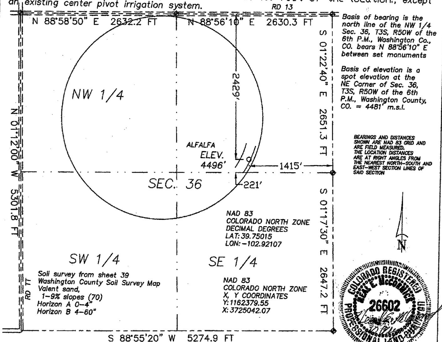
Basis of bearing is the north line of the NW 1/4 Sec. 36, T3S, R50W of the 6th P.M., Washington Co., CO. bears N 88°56'10" E between set monuments
