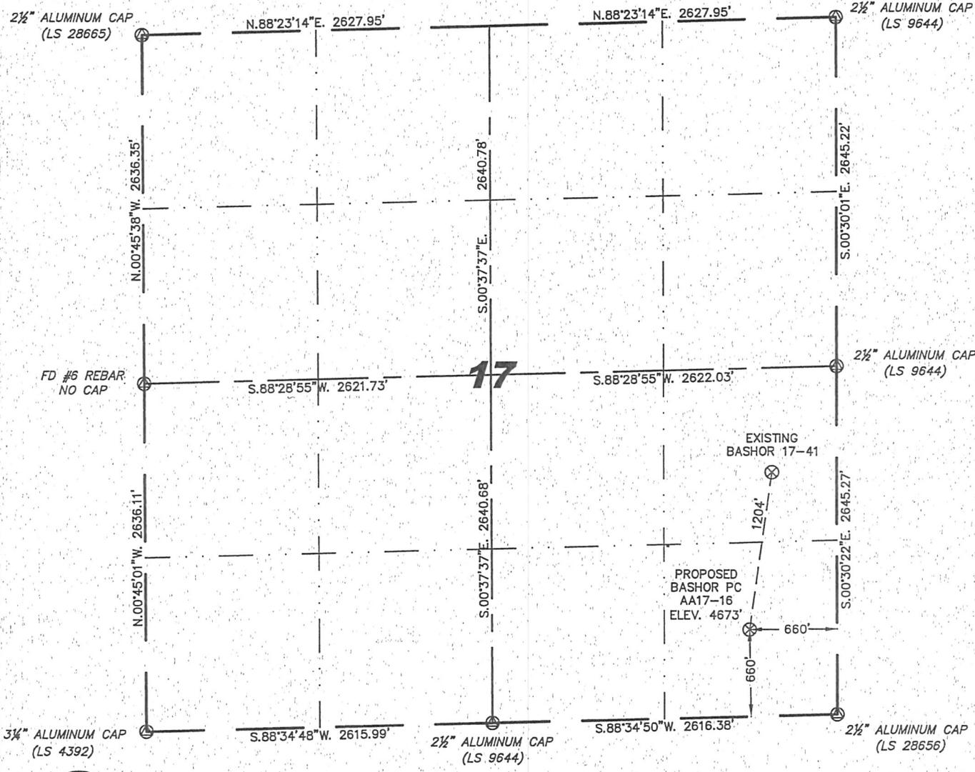
IN ACCORDANCE WITH A REQUEST FROM ERIK VAN DECAR - NOBLE ENERGY INC. STEIL SURVEYING SERVICES, LLC HAS DETERMINED THE LOCATION OF THE BASHOR PC AA17-16 WELL TO BE 660' FSL, 660' FEL, AS MEASURED AT NINETY (90) DEGREES FROM THE SECTION LINES, SECTION 17, TOWNSHIP 6 NORTH, RANGE 63 WEST, 6TH PRINCIPLE MERIDIAN, WELD COUNTY, COLORADO.
