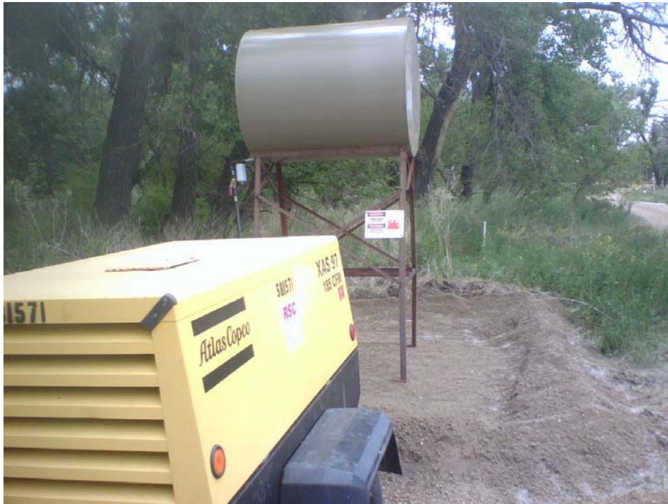
Photo 1: Air sparging system with a diesel-powered air compressor. Fuel tank is bermed.
