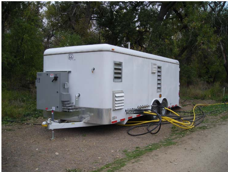
Photo:2 Air sparging/soil vapor extraction system trailer. Components are housed in a trailer for versatility and ease of transport to treat multiple sites.
