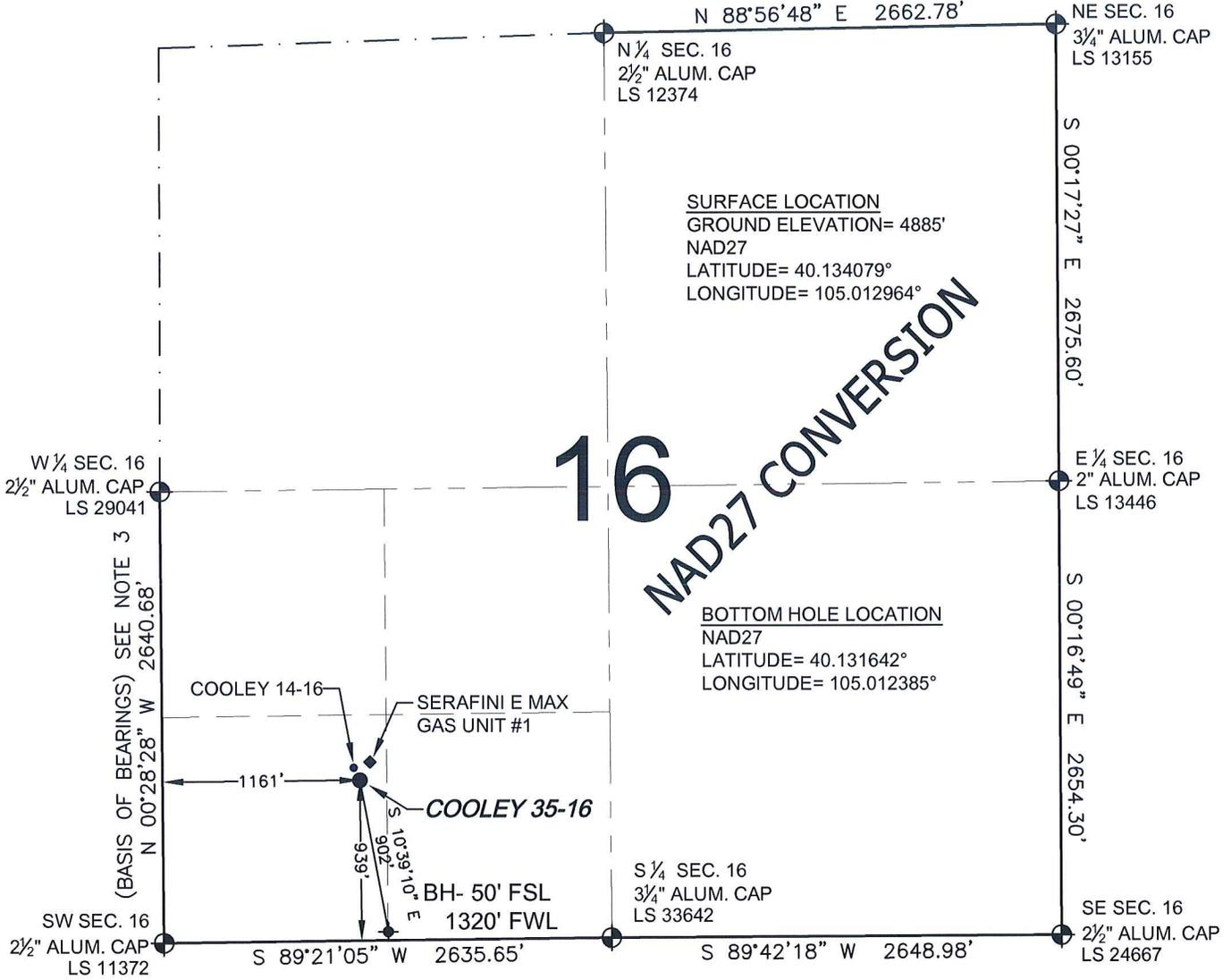
WELL **COOLEY 35-16** TO BE LOCATED 939' FSL AND 1161' FWL, SECTION 16, T2N, R68W OF THE 6th P.M.
