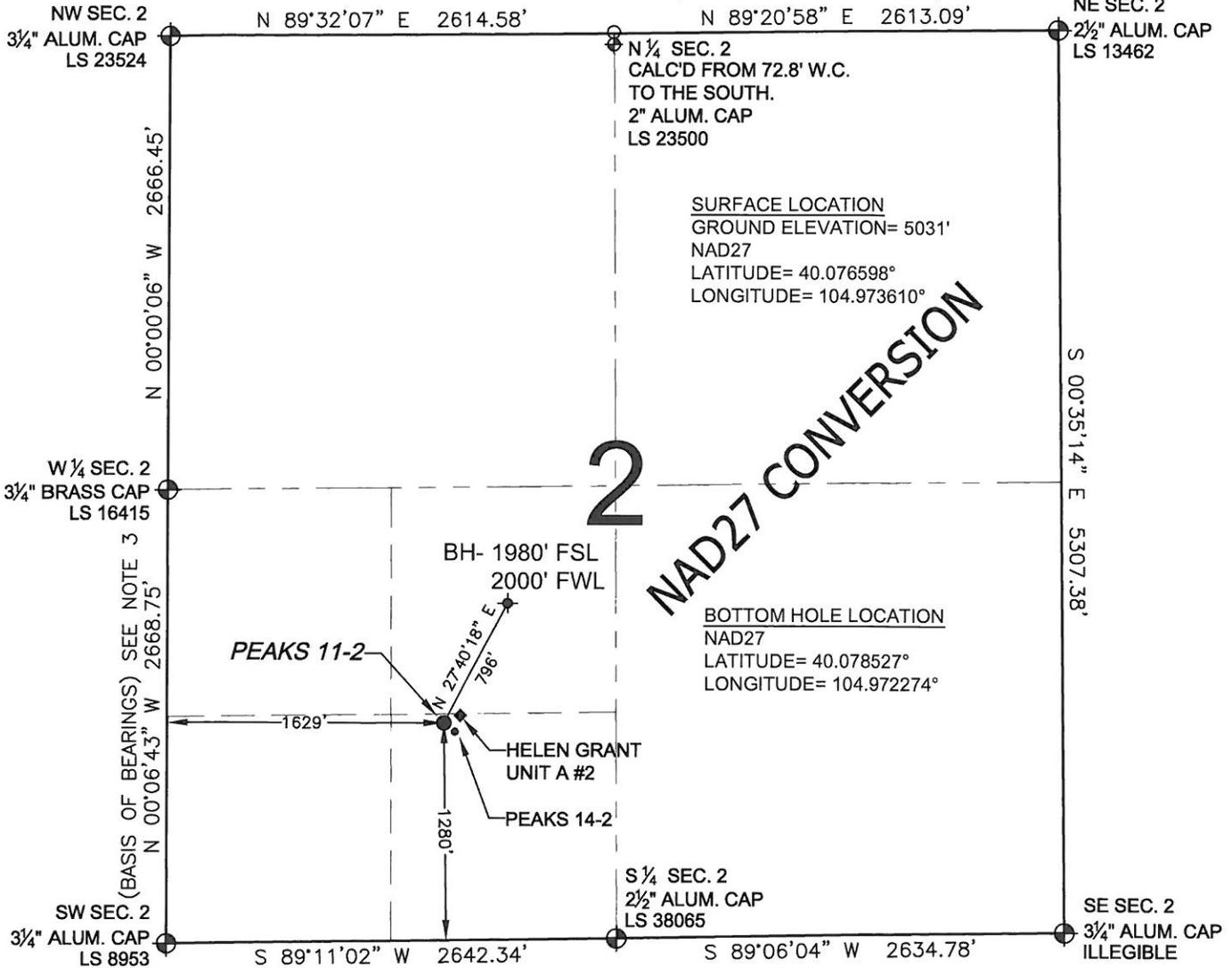
WELL PEAKS 11-2 TO BE LOCATED 1280' FSL AND 1629' FWL, SECTION 2, T1N, R68W OF THE 6th P.M.
