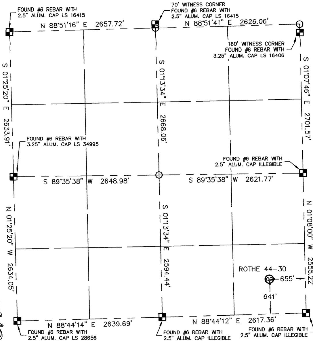
In accordance with a request from JARED RUSH with Texas American Resources Co. Lat40°, LLC has determined the surface location of the ROTHE 44-30 to be 641' from the SOUTH line and 655' from the EAST line as measured at right angles from the section line of Section 30, Township 5 North, Range 63 West of the Sixth Principal Meridian, County of Weld, State of Colorado.
