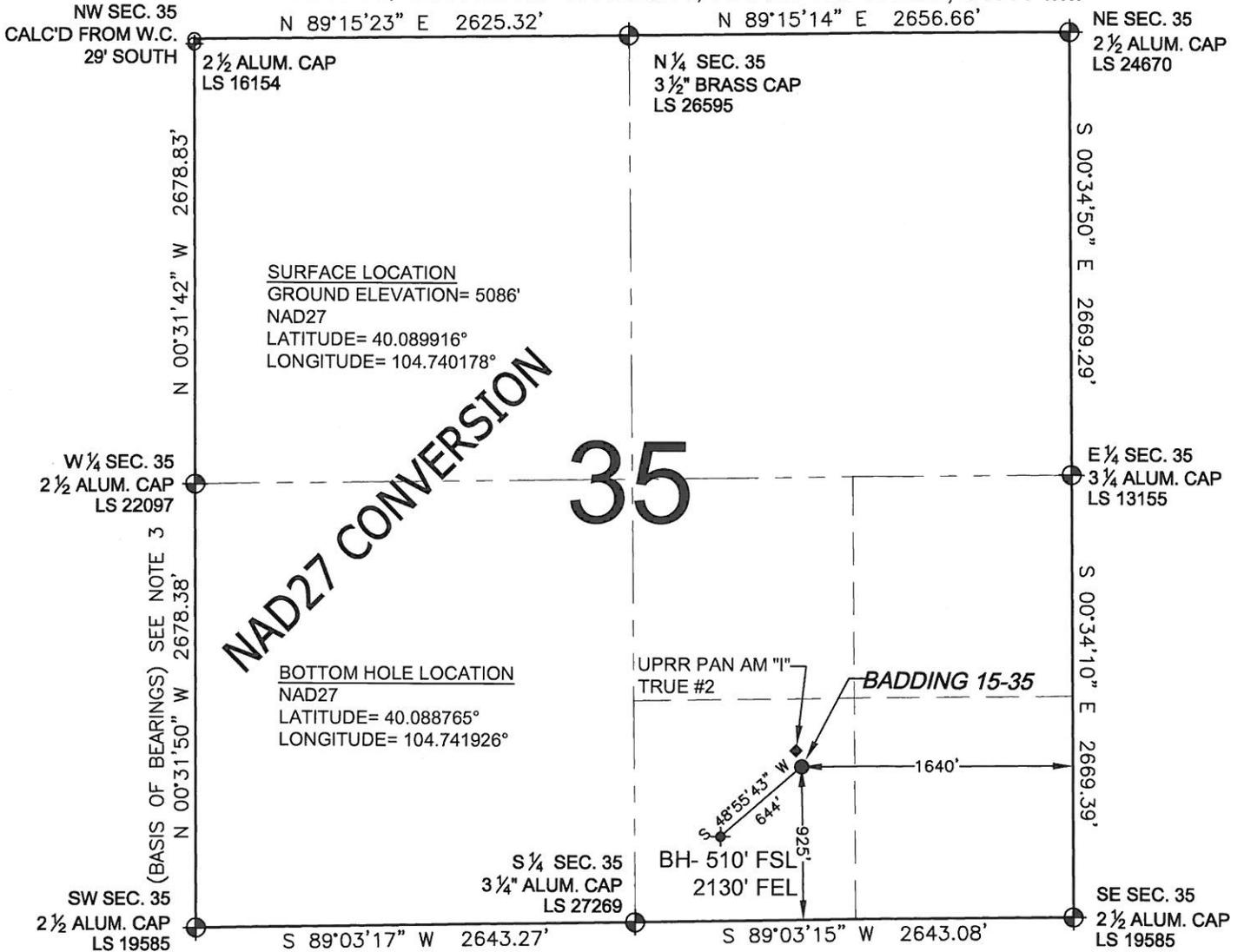
WELL **BADDING 15-35** TO BE LOCATED 925' FSL AND 1640' FEL, SECTION 35, T2N, R66W OF THE 6th P.M.
