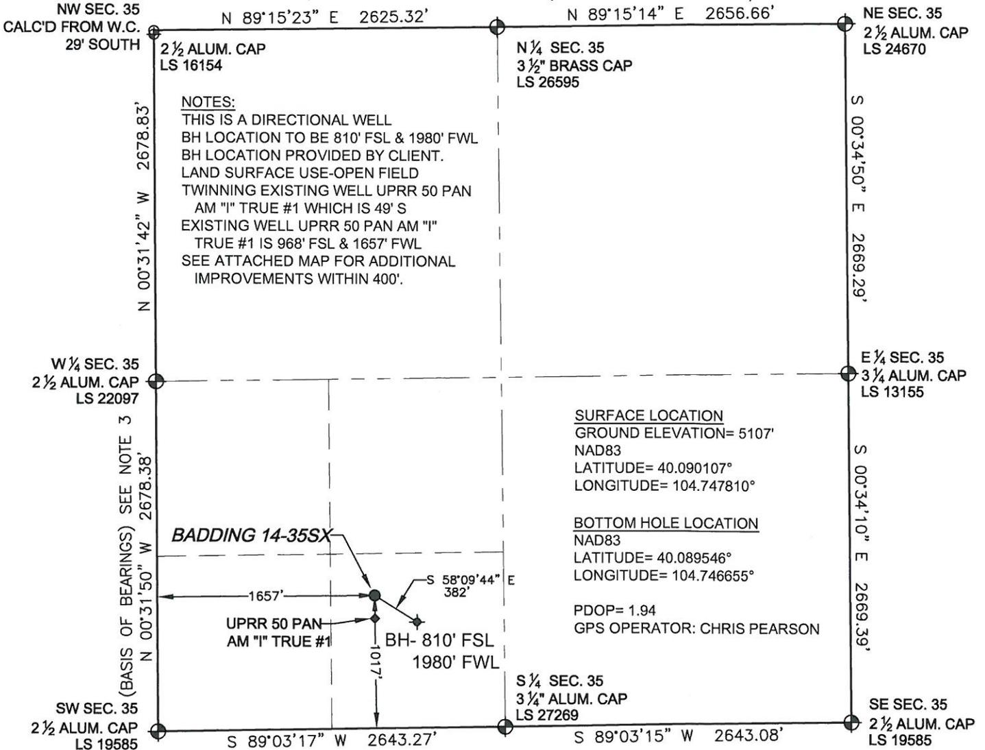
WELL **BADDING 14-35SX** TO BE LOCATED 1017' FSL AND 1657' FWL, SECTION 35, T2N, R66W OF THE 6th P.M.
