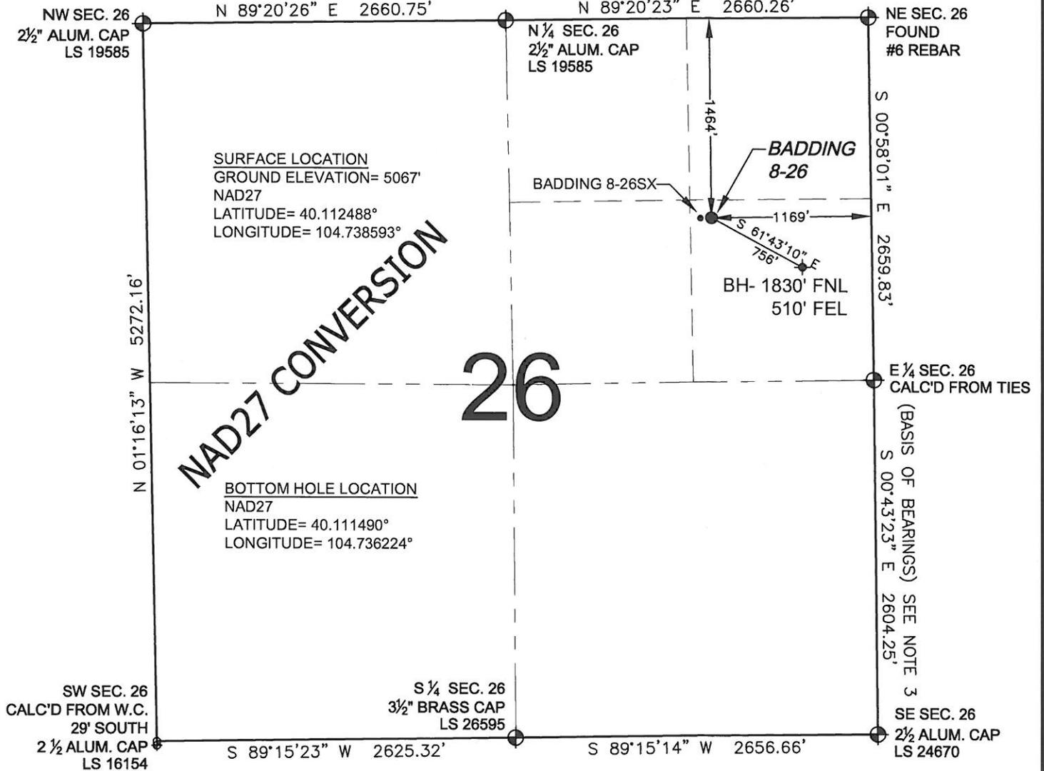
WELL **BADDING 8-26** TO BE LOCATED 1464' FNL AND 1169' FEL, SECTION 26, T2N, R66W OF THE 6th P.M.
