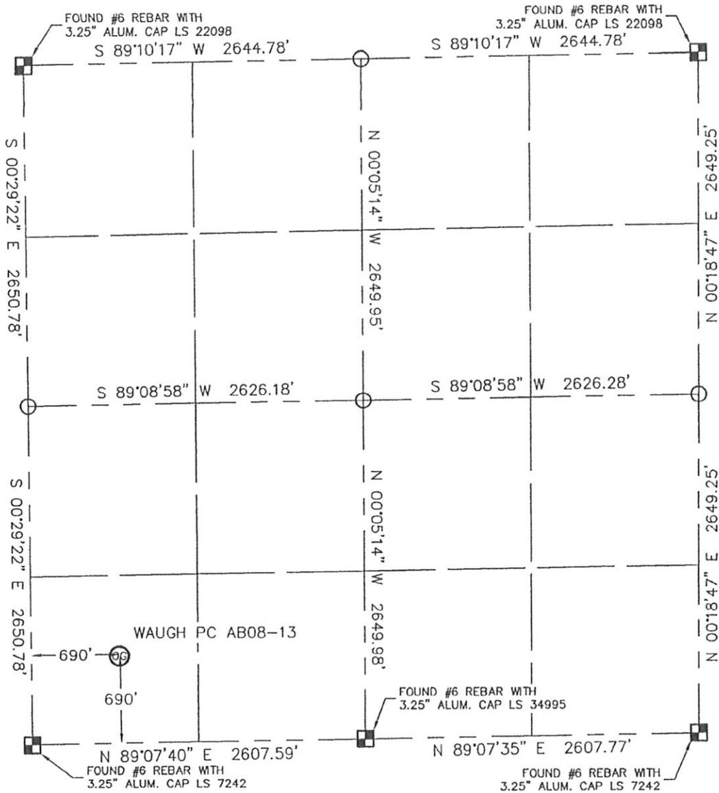
In accordance with a request from RYAN ANTONIO with Noble Energy Inc., Lat40°, LLC has determined the surface location of the WAUGH PC AB08-13 to be 690' from the SOUTH line and 690' from the WEST line as measured at right angles from the section line of Section 8, Township 7 North, Range 64 West of the Sixth Principal Meridian, County of Weld, State of Colorado.
