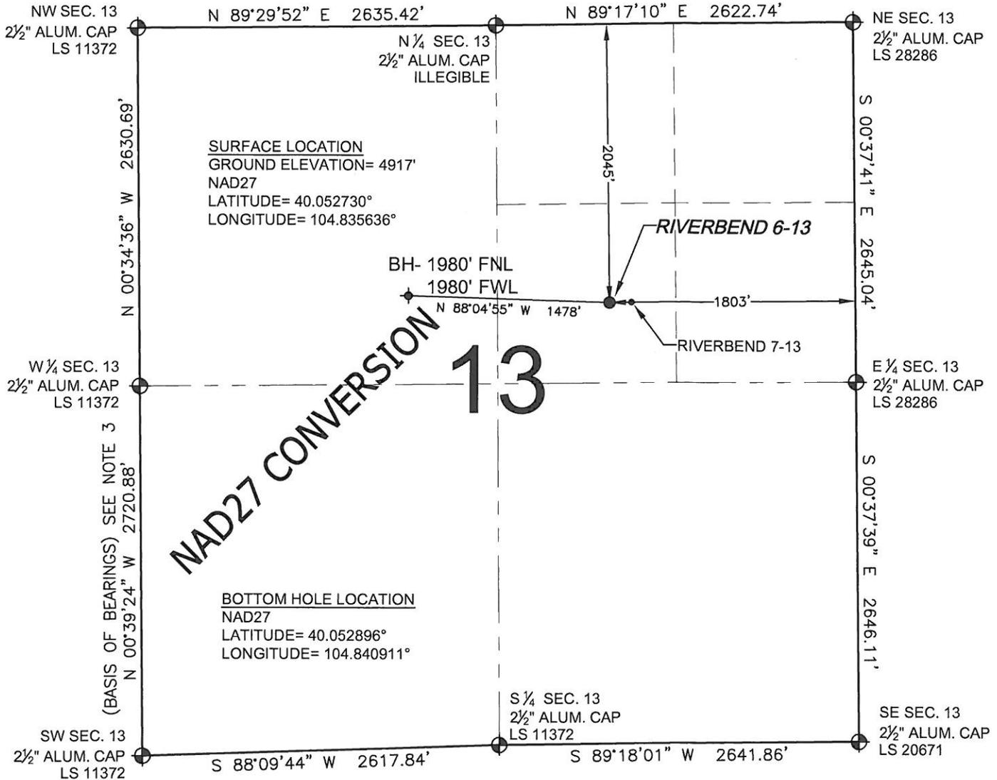
WELL **RIVERBEND 6-13** TO BE LOCATED 2045' FNL AND 1803' FEL, SECTION 13, T1N, R67W OF THE 6th P.M.
