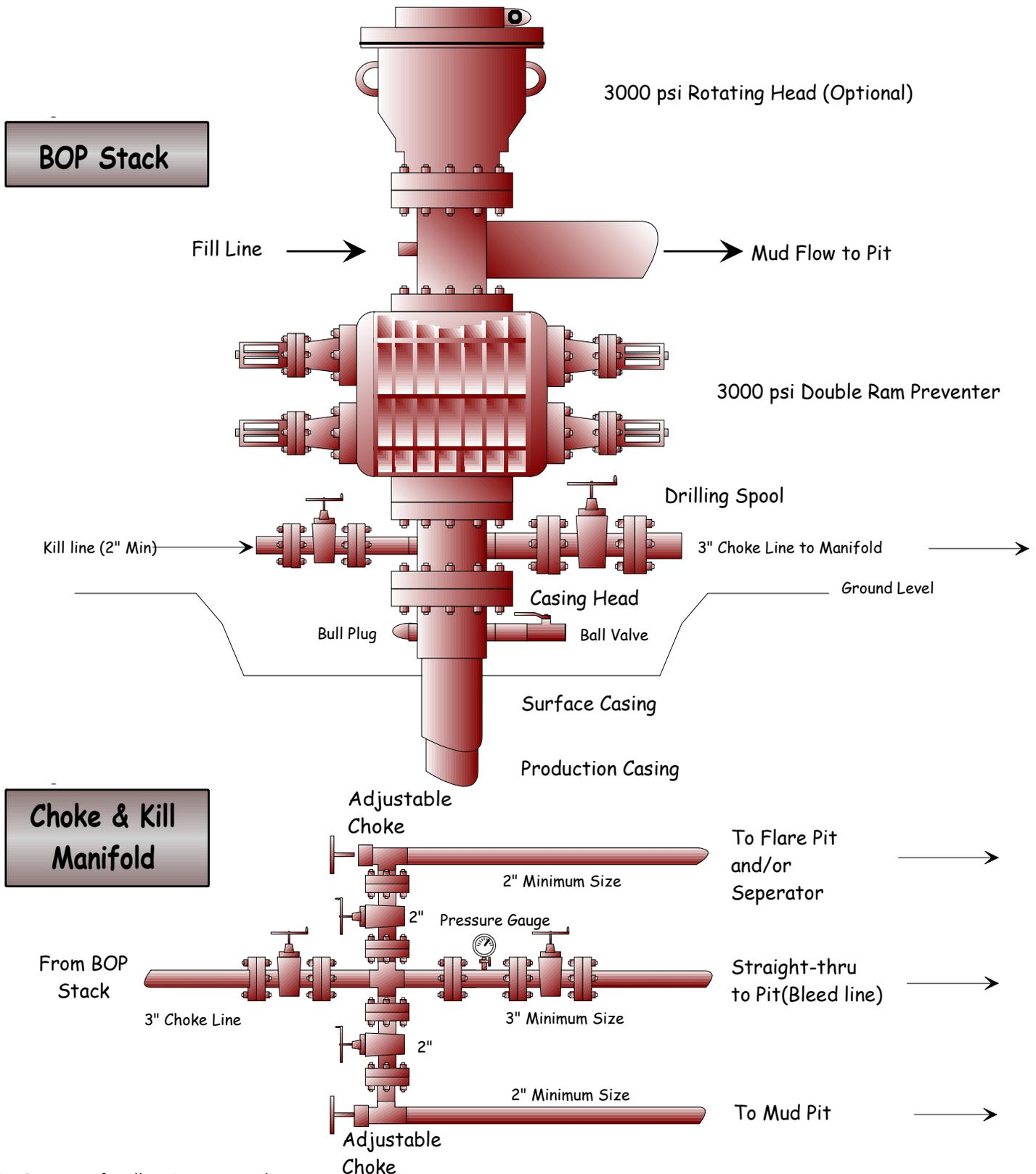
Working Pressures for all equipment, Annular Preventor and both rams are rated to 3000 psi or greater
