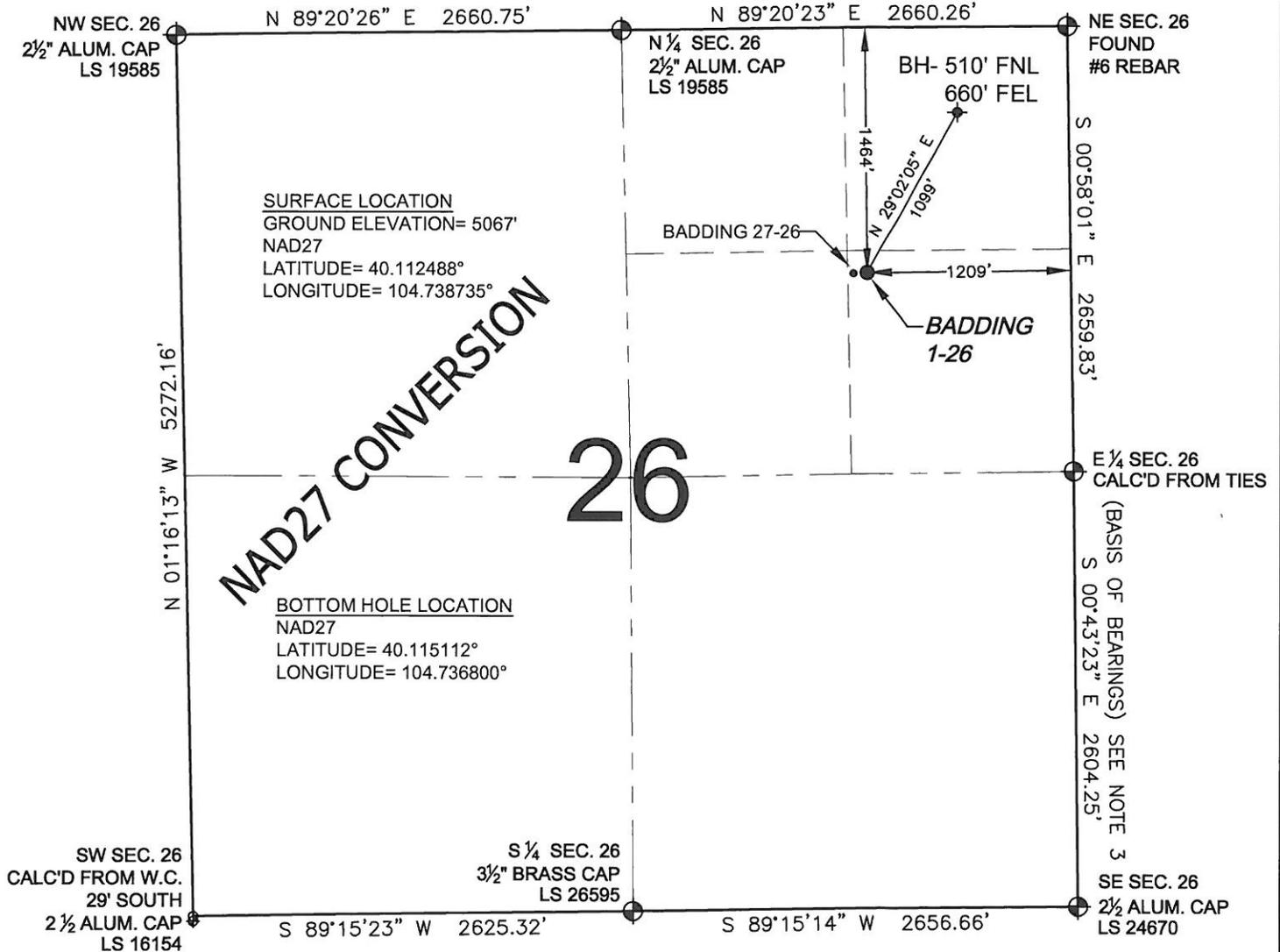
WELL **BADDING 1-26** TO BE LOCATED 1464' FNL AND 1209' FEL, SECTION 26, T2N, R66W OF THE 6th P.M.
