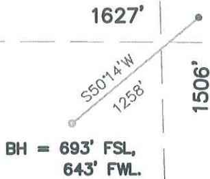
I HEREBY STATE TO UNIOIL THAT THIS WELL LOCATION CERTIFICATE FOR THE WELL WEDCO 14-21DU IS LOCATED 1506' FSL & 1627' FWL, SEC. 21, T4N, R67W, 6PM.
