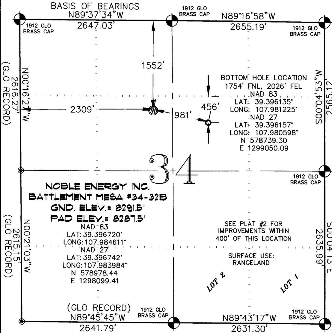
THIS WELL LOCATION PLAT WAS PREPARED FOR NOBLE ENERGY INC. TO LOCATE THE BATTLEMENT MESA #34-32B WELL, 1552 FEET FROM THE NORTH LINE AND 2309 FEET FROM THE WEST LINE IN THE SE1/4 NW1/4 OF SECTION 34, T. 7 S., R. 95 W. OF THE 6TH P.M. GARFIELD COUNTY, COLORADO.
