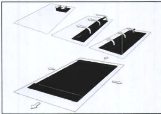
2. Next, locate the spill berm. Unfold the spill berm and center it on top of the ground cover.
