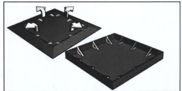
For the InstaBerm, pull all four sidewalls of the spill berm outward so that they are standing upright. Straighten the top angles of the wall supports inside the berm. The walls will move further outward as the berm is filled.
