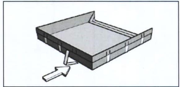
For the bracketed berm, locate the aluminum angle brackets. Insert the angle brackets into the perimeter pockets on three sides of the spill berm. Use the unsupported end for equipment entry. After equipment is in place, insert the angle brackets on the fourth side to complete the installation.
