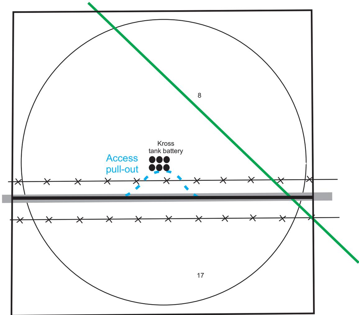
Pull-out will have culvert placed, then barrow ditch filled with road-base.
