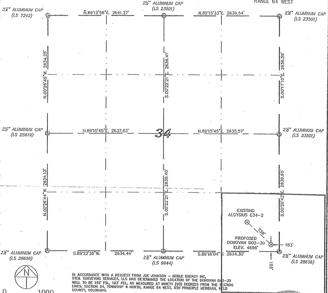
IN ACCORDANCE WITH A REQUEST FROM JOE JOHNSON - NOBLE ENERGY INC, STEIL SURVEYING SERVICES, LLC HAS DETERMINED THE LOCATION OF THE DONOVAN D02-30 WELL TO BE 155' FSL, 183' FEL, AS MEASURED AT NINETY (90) DEGREES FROM THE SECTION LINES, SECTION 34, TOWNSHIP 4 NORTH, RANGE 64 WEST, 6TH PRINCIPLE MERIDIAN, WELD COUNTY, COLORADO.
