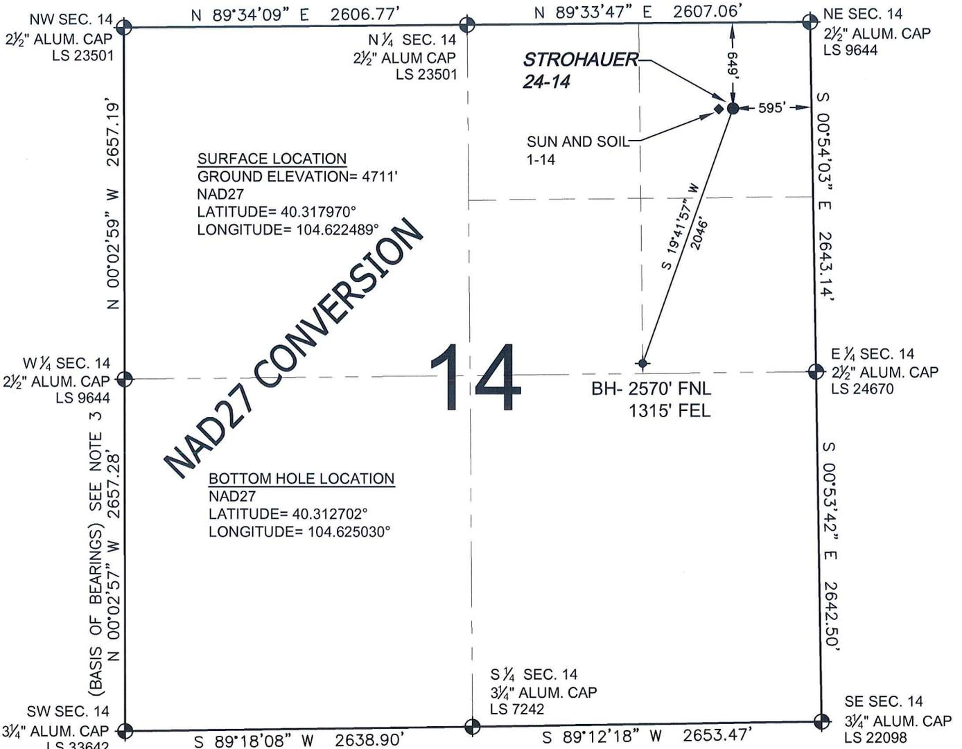
WELL **STROHAUER 24-14** TO BE LOCATED 649' FNL AND 595' FEL, SECTION 14, T4N, R65W OF THE 6th P.M.
