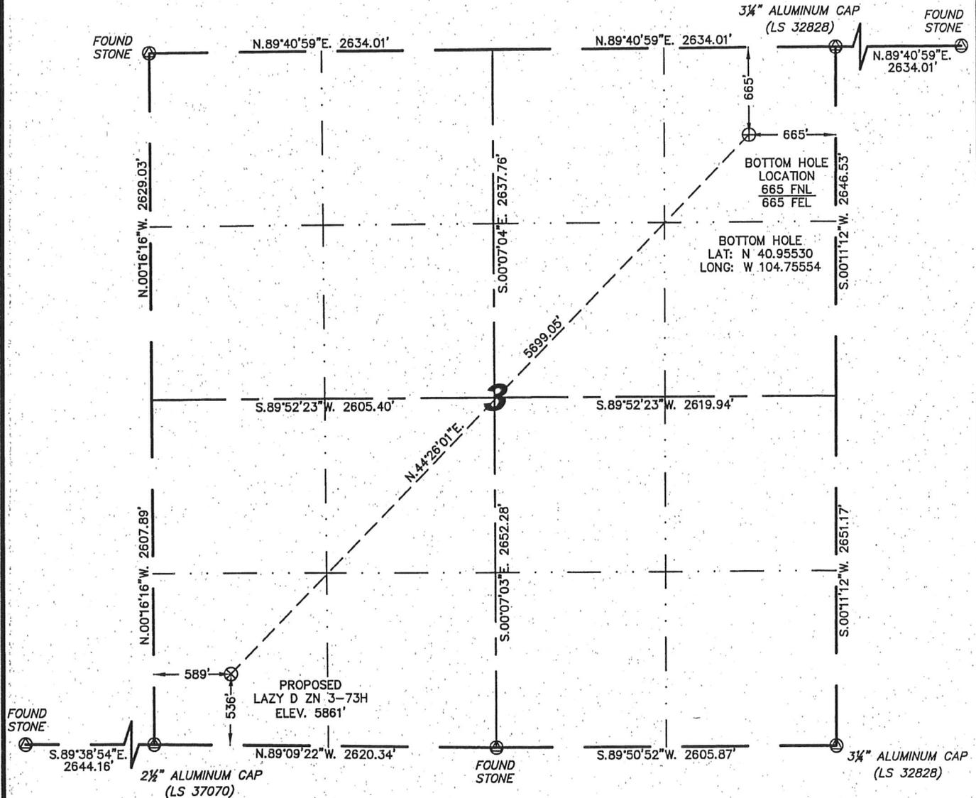
IN ACCORDANCE WITH A REQUEST FROM DIRK SWARTZ - NOBLE ENERGY INC, STEIL SURVEYING SERVICES, LLC HAS DETERMINED THE LOCATION OF THE LAZY D ZN 3-73H WELL TO BE 536' FSL, 589' FWL, AS MEASURED AT NINETY (90) DEGREES FROM THE SECTION LINES, SECTION 3, TOWNSHIP 11 NORTH, RANGE 66 WEST, 6TH PRINCIPLE MERIDIAN, WELD COUNTY, COLORADO.
