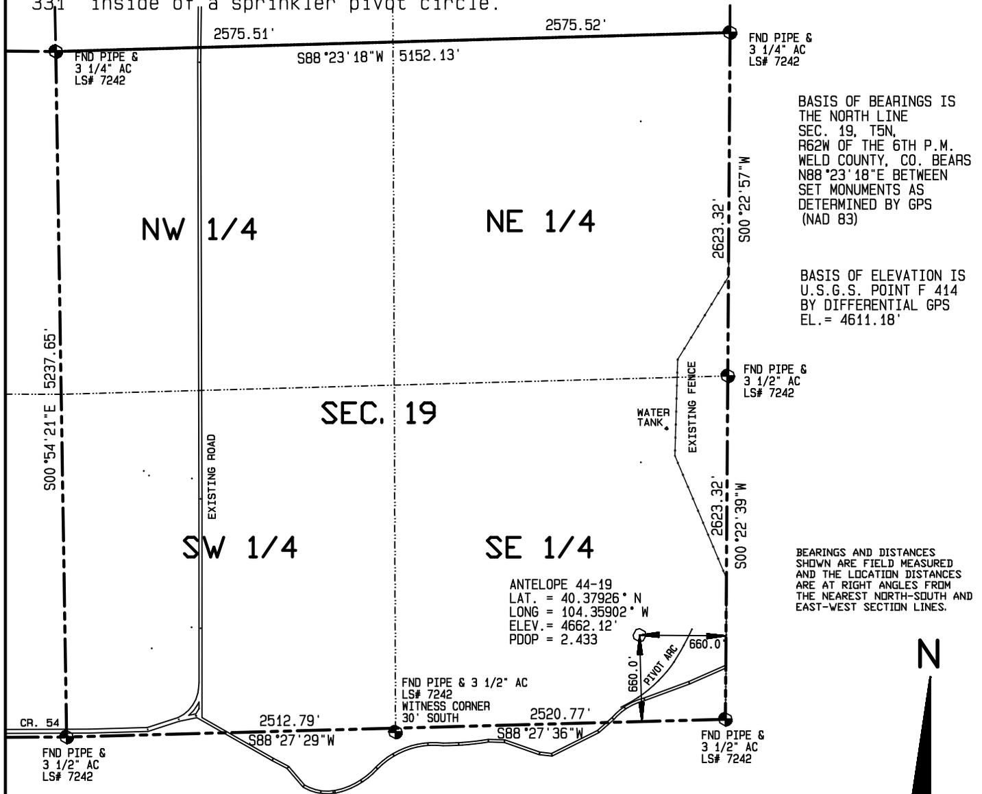
BASIS OF BEARINGS IS THE NORTH LINE SEC. 19, T5N, R62W OF THE 6TH P.M. WELD COUNTY, CO. BEARS N88°23'18\"E BETWEEN SET MONUMENTS AS DETERMINED BY GPS (NAD 83)
