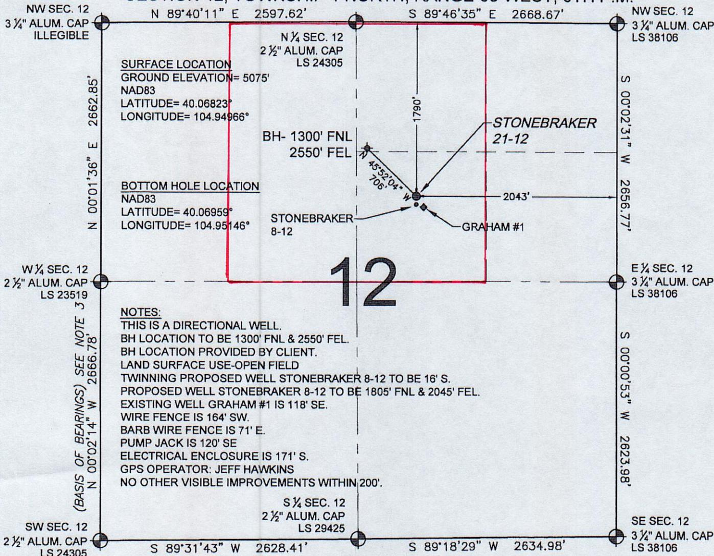
WELL **STONEBRAKER 21-12** TO BE LOCATED 1790' FNL AND 2043' FEL, SECTION 12, T1N, R68W OF THE 6th P.M.
