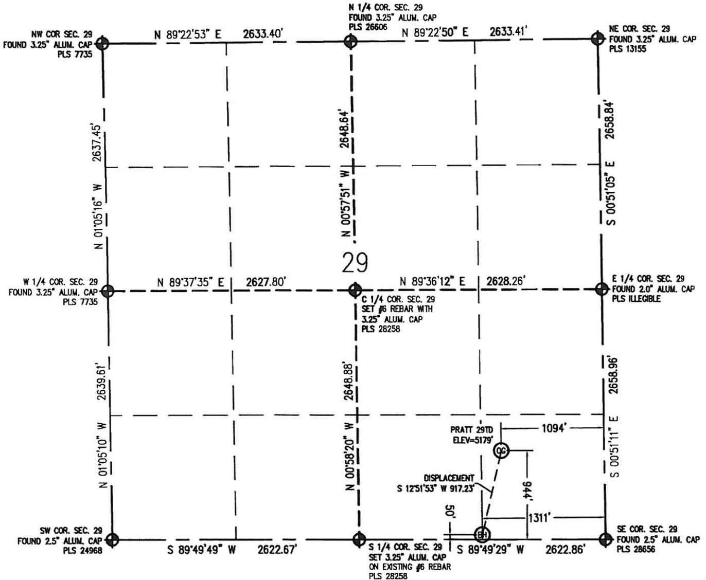
IN ACCORDANCE WITH A REQUEST FROM CRAIG RASMUSON - SYNERGY RESOURCES, BASELINE ENGINEERING CORP. HAS DETERMINED THE LOCATION OF THE PRATT 29TD TO BE 944' FSL AND 1094' FEL, AS MEASURED AT NINETY (90) DEGREES FROM THE SECTION LINE OF SECTION 29, TOWNSHIP 1 NORTH, RANGE 68 WEST AND THE BOTTOM HOLE LOCATION TO BE 50' FSL AND 1311' FEL OF SECTION 29, TOWNSHIP 1 NORTH, RANGE 68 WEST, 6TH PRINCIPAL MERIDIAN, WELD COUNTY, COLORADO.
