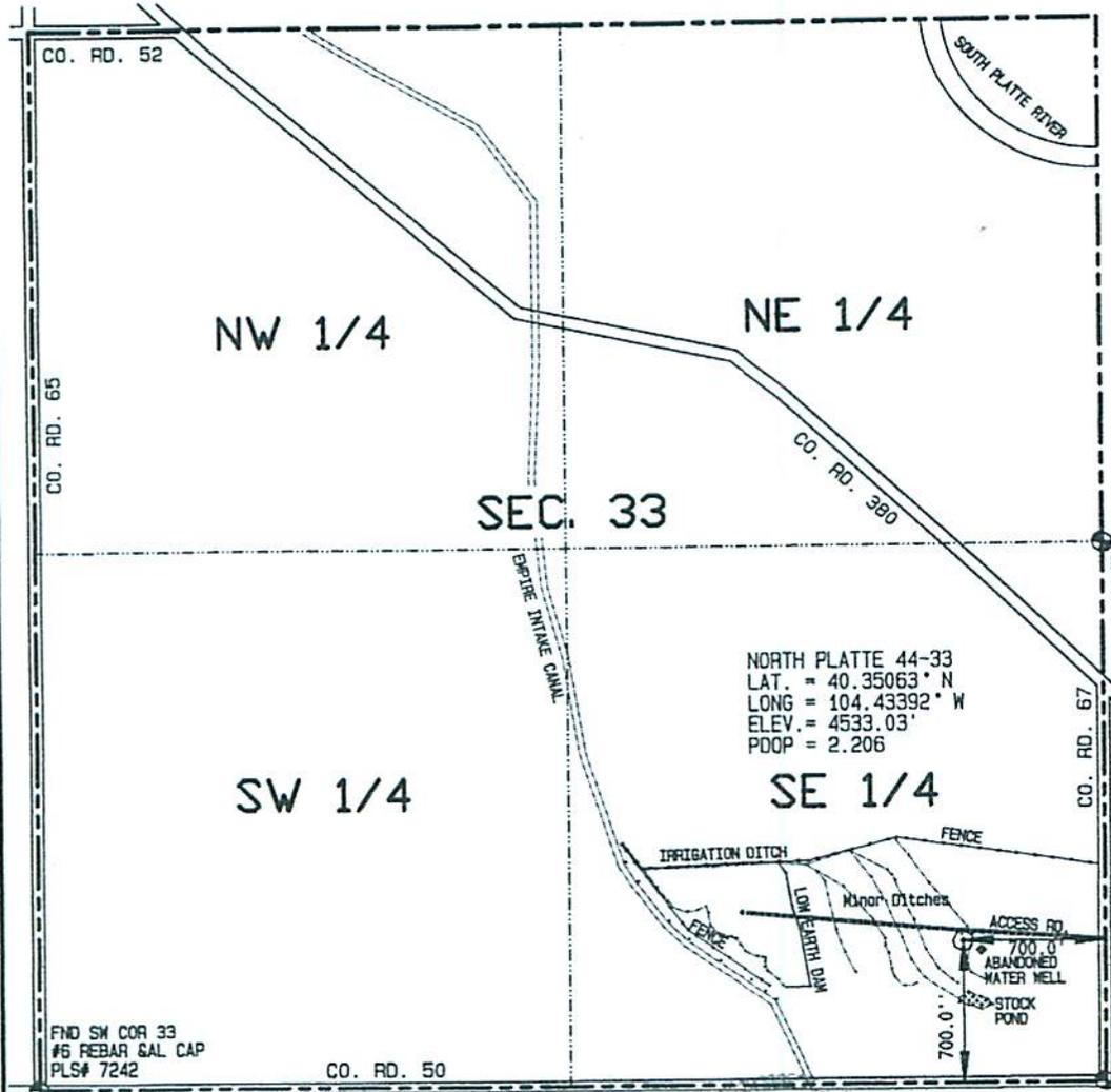
BASIS OF BEARINGS IS THE SOUTH LINE OF SEC. 33, T5N, R63W OF THE 6TH P.M. WELD COUNTY, CO. BEARS S89°54'07\"/>
