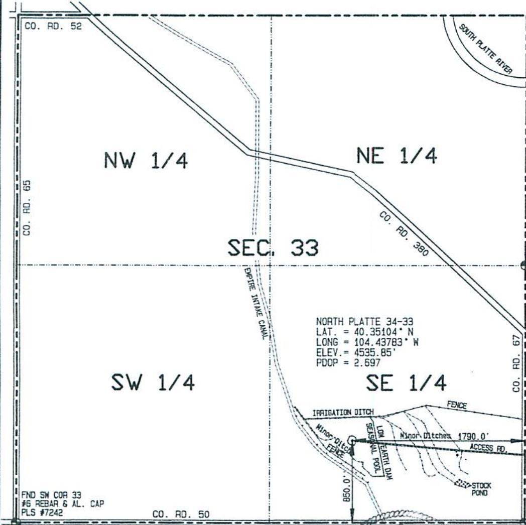
BASIS OF BEARINGS IS THE SOUTH LINE OF SEC. 33, T5N, R63W OF THE 6TH P.M. WELD COUNTY, CO. BEARS S89°54'07"E BETWEEN SET MONUMENTS AS DETERMINED BY GPS (NAD 83)
