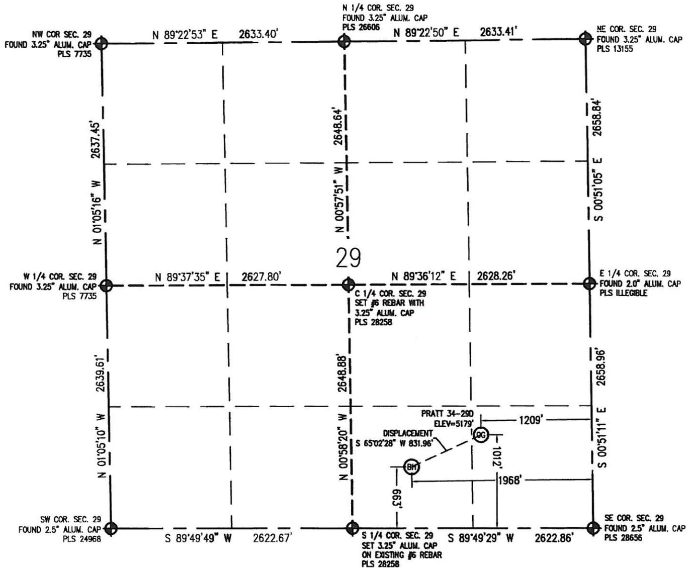
IN ACCORDANCE WITH A REQUEST FROM CRAIG RASMUSON - SYNERGY RESOURCES, BASELINE ENGINEERING CORP. HAS DETERMINED THE LOCATION OF THE PRATT 34-29D TO BE 1012' FSL AND 1209' FEL, AS MEASURED AT NINETY (90) DEGREES FROM THE SECTION LINE OF SECTION 29, TOWNSHIP 1 NORTH, RANGE 68 WEST AND THE BOTTOM HOLE LOCATION TO BE 663' FSL AND 1968' FEL OF SECTION 29, TOWNSHIP 1 NORTH, RANGE 68 WEST, 6TH PRINCIPAL MERIDIAN, WELD COUNTY, COLORADO.
