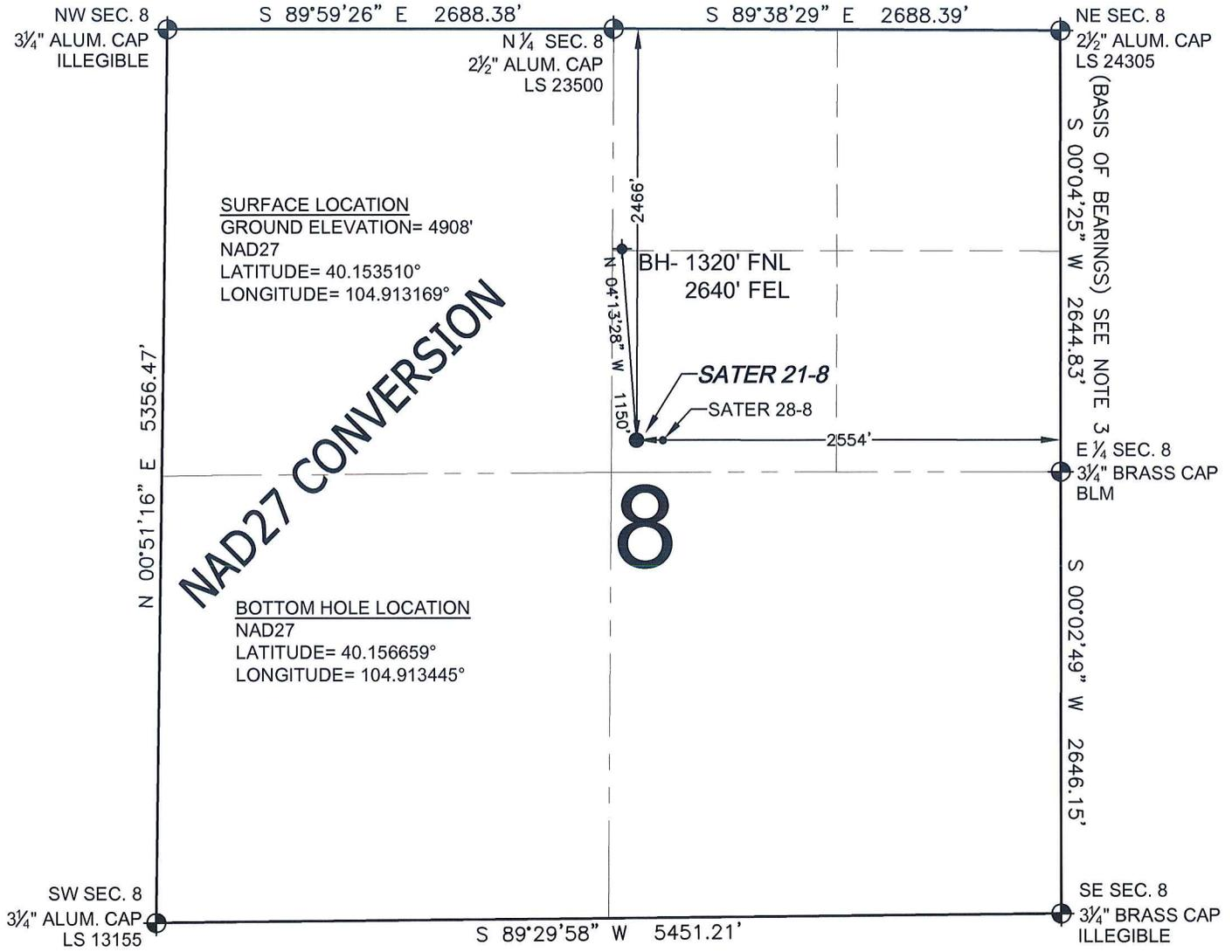
WELL **SATER 21-8** TO BE LOCATED 2466' FNL AND 2554' FEL, SECTION 8, T2N, R67W OF THE 6th P.M.
