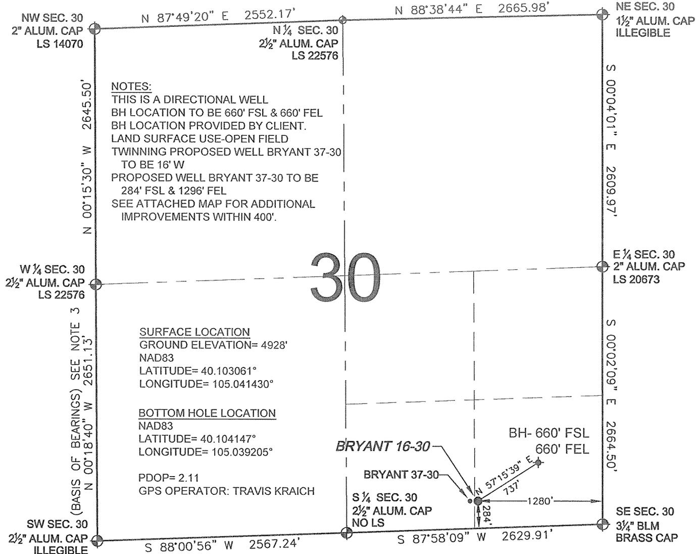
WELL **BRYANT 16-30** TO BE LOCATED 284' FSL AND 1280' FEL, SECTION 30, T2N, R68W OF THE 6th P.M.
