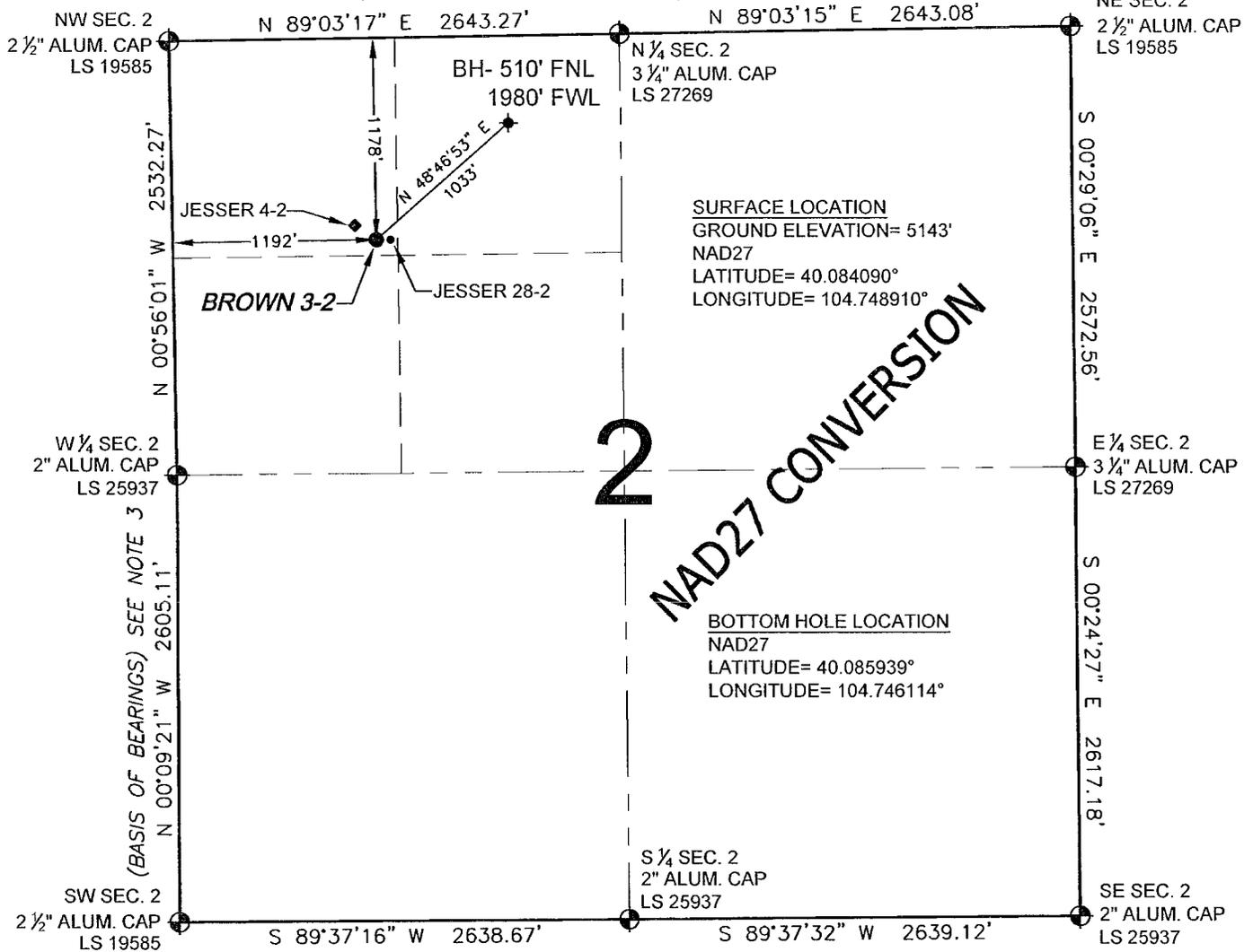
WELL **BROWN 3-2** TO BE LOCATED 1178' FNL AND 1192' FWL, SECTION 2, T1N, R66W OF THE 6th P.M.
