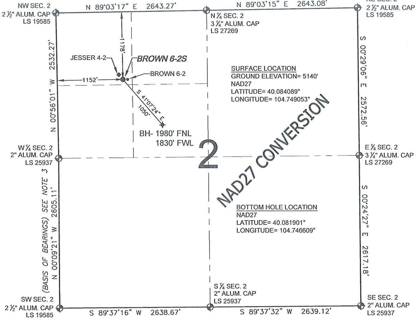
WELL **BROWN 6-2S** TO BE LOCATED 1178' FNL AND 1152' FWL, SECTION 2, T1N, R66W OF THE 6th P.M.
