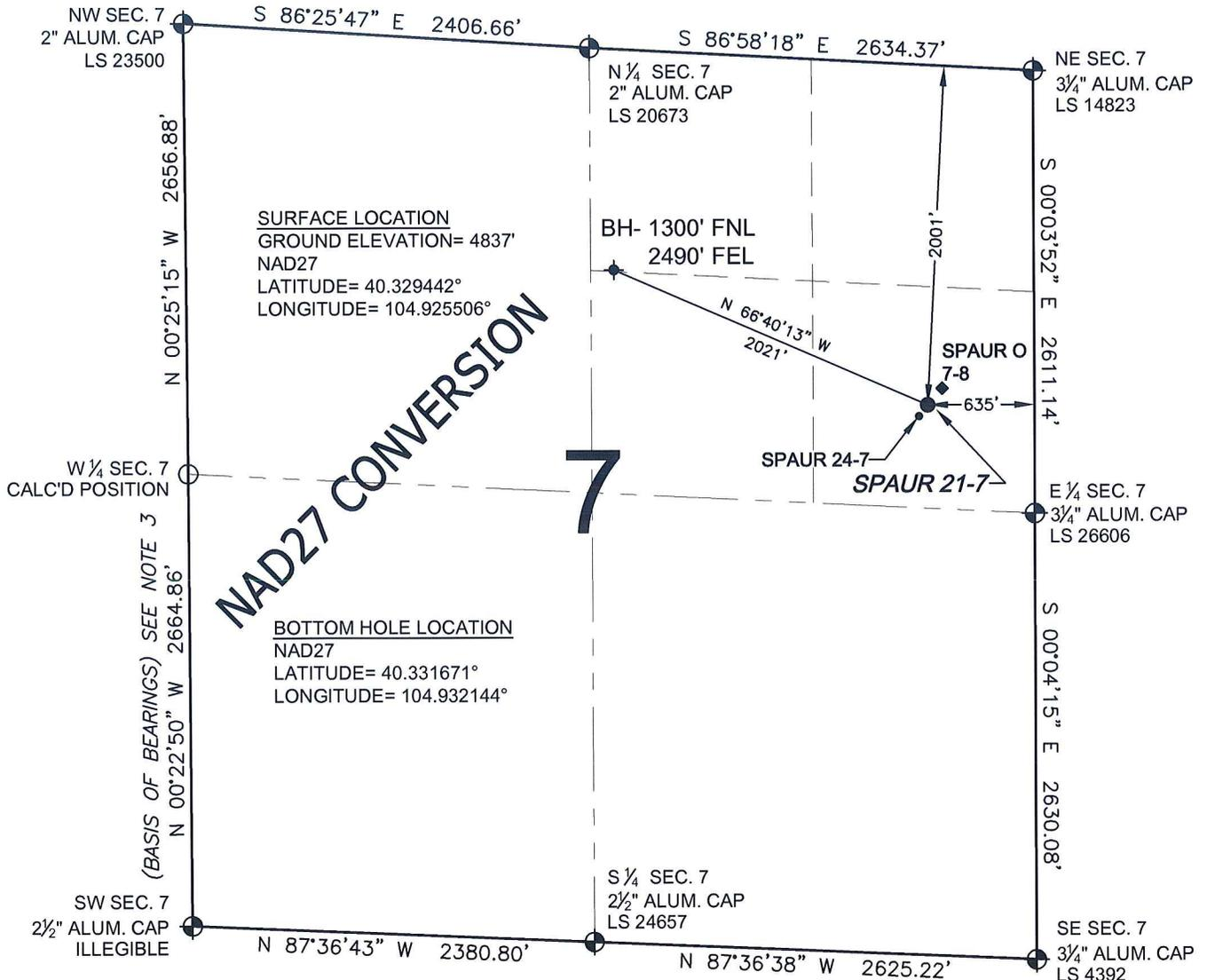
WELL SPAUR 21-7 TO BE LOCATED 2001' FNL AND 635' FEL, SECTION 7, T4N, R67W OF THE 6th P.M.
