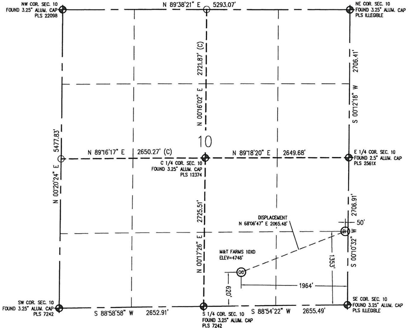
IN ACCORDANCE WITH A REQUEST FROM CRAIG RASMUSON - SYNERGY RESOURCES, BASELINE ENGINEERING CORP. HAS DETERMINED THE LOCATION OF THE M&T FARMS 10XD TO BE 620' FSL AND 1964' FEL, AS MEASURED AT NINETY (90) DEGREES FROM THE SECTION LINE OF SECTION 10, TOWNSHIP 6 NORTH, RANGE 65 WEST AND THE BOTTOM HOLE LOCATION TO BE 1353' FSL AND 50' FEL OF SECTION 10, TOWNSHIP 6 NORTH, RANGE 65 WEST, 6TH PRINCIPAL MERIDIAN, WELD COUNTY, COLORADO.
