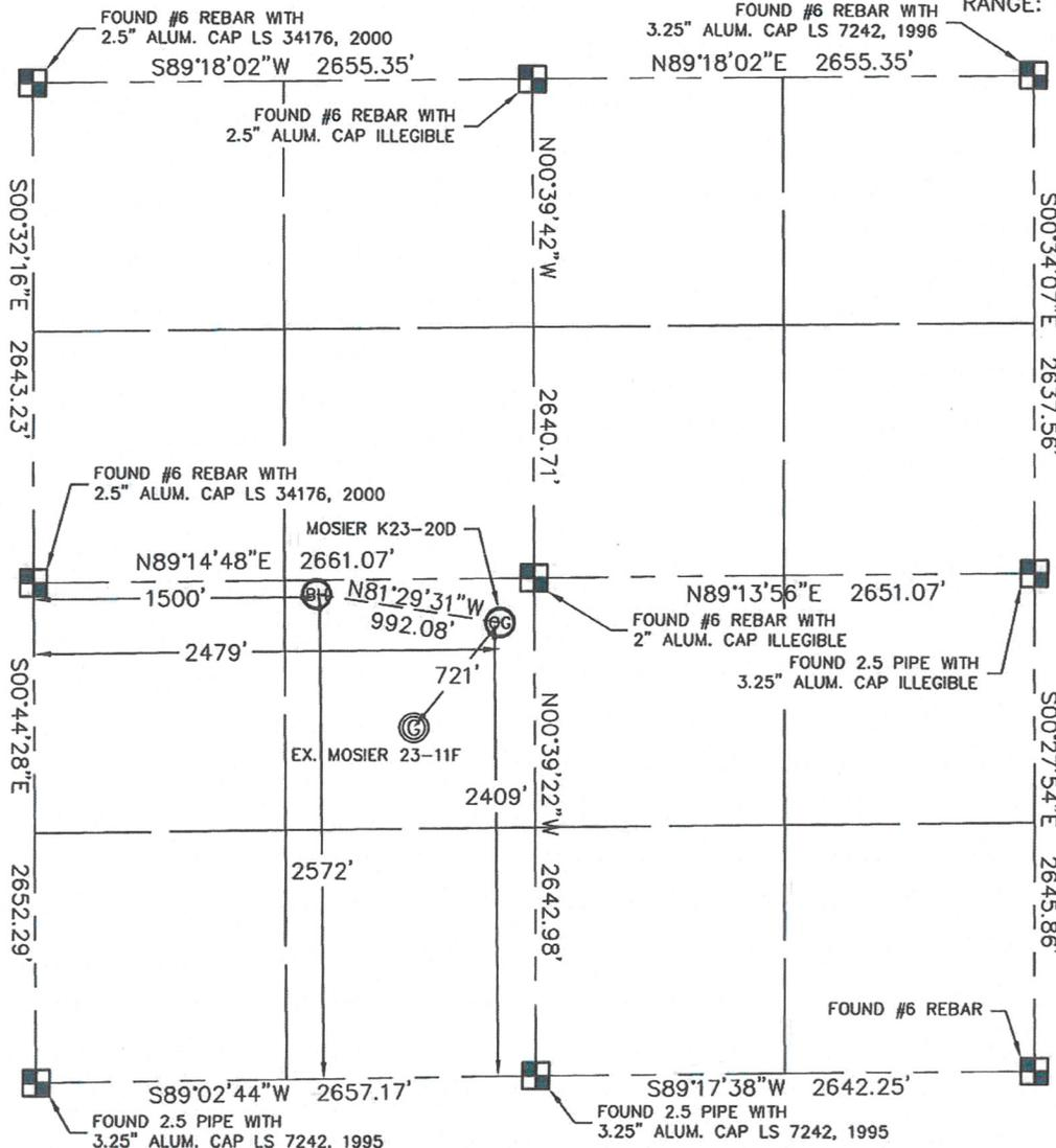
In accordance with a request from **JOE MARTIN** with **Noble Energy Inc.** King Surveyors Inc. has determined the surface location of the **MOSIER K23-20D** to be 2409' from the SOUTH line and 2479' from the WEST line and the bottom hole to be 2572' from the SOUTH line and 1500' from the WEST line as measured at right angles from the section line of **Section 23, Township 4 North, Range 66 West** of the Sixth Principal Meridian, County of Weld, State of Colorado.
