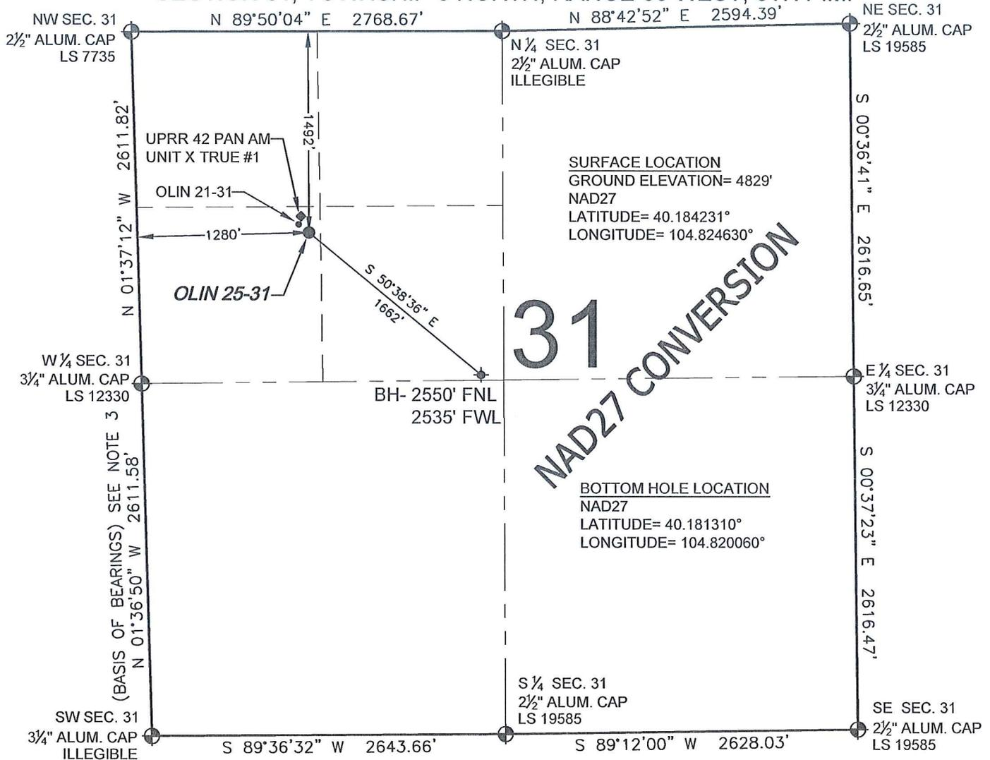
WELL **OLIN 25-31** TO BE LOCATED 1492' FNL AND 1280' FWL, SECTION 31, T3N, R66W OF THE 6th P.M.
