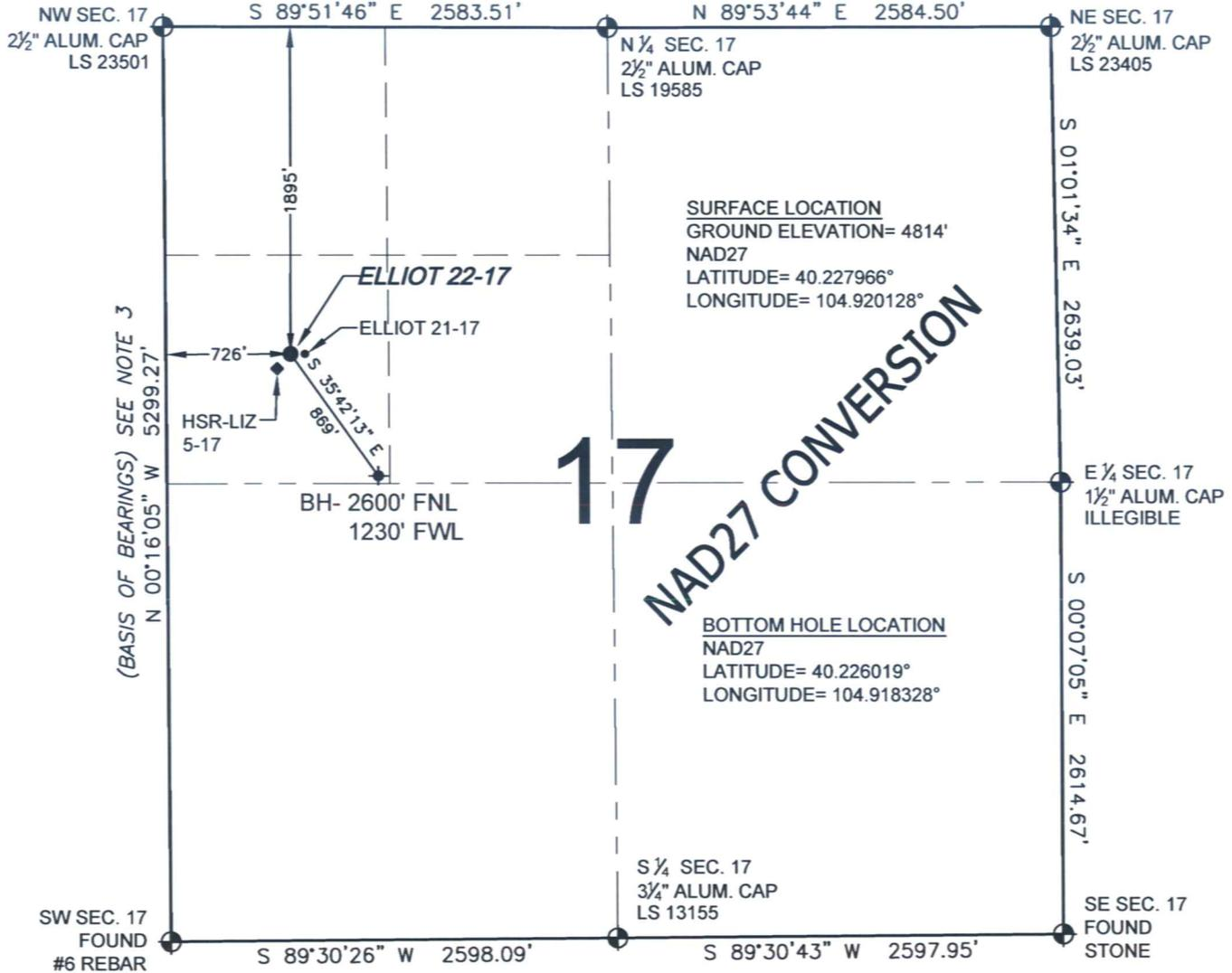
WELL ELLIOT 22-17 TO BE LOCATED 1895' FNL AND 726' FWL, SECTION 17, T3N, R67W OF THE 6th P.M.
