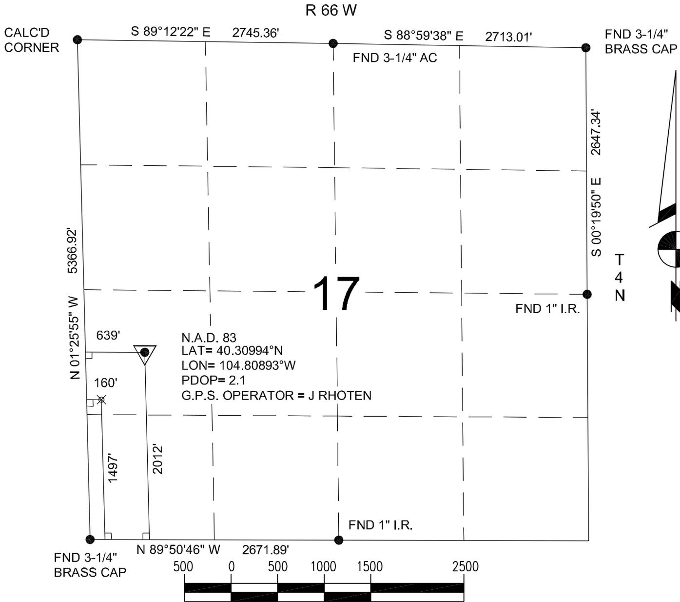
Power Surveying Co., Inc. of Frederick, Colorado has in accordance with a request from SHERRY GLASS for KP KAUFFMAN CO. determined the location of FRONT RANGE 12-17-33 to be 2012' FSL & 639' FWL Section 17, Township 4 NORTH Range 66 WEST of the Sixth Principal Meridian, WELD County, COLORADO
