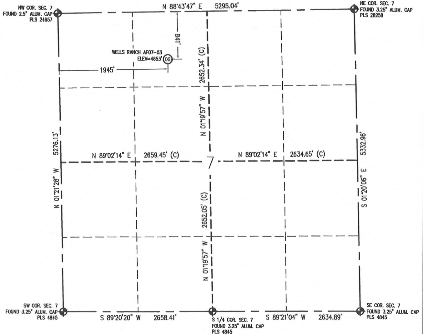
IN ACCORDANCE WITH A REQUEST FROM SEAN CASPER – NOBLE ENERGY, BASELINE ENGINEERING CORP. HAS DETERMINED THE LOCATION OF THE WELLS RANCH AF07-03 TO BE 841' FNL AND 1945' FWL, AS MEASURED AT NINETY (90) DEGREES FROM THE SECTION LINE OF SECTION 7, TOWNSHIP 5 NORTH, RANGE 62 WEST, 6TH PRINCIPAL MERIDIAN, WELD COUNTY, COLORADO.
