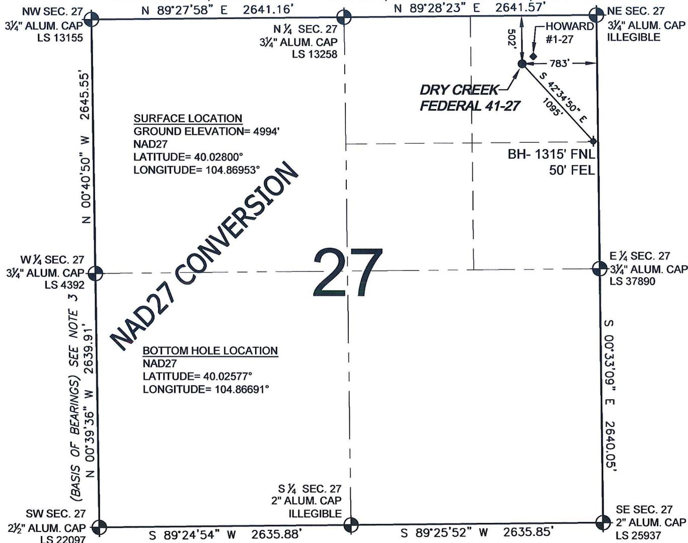
WELL DRY CREEK FEDERAL 41-27 TO BE LOCATED 502' FNL AND 783' FEL, SECTION 27, T1N, R67W OF THE 6th P.M.
