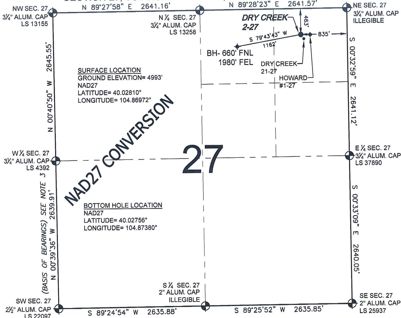
WELL **DRY CREEK 2-27** TO BE LOCATED 463' FNL AND 835' FEL, SECTION 27, T1N, R67W OF THE 6th P.M.
