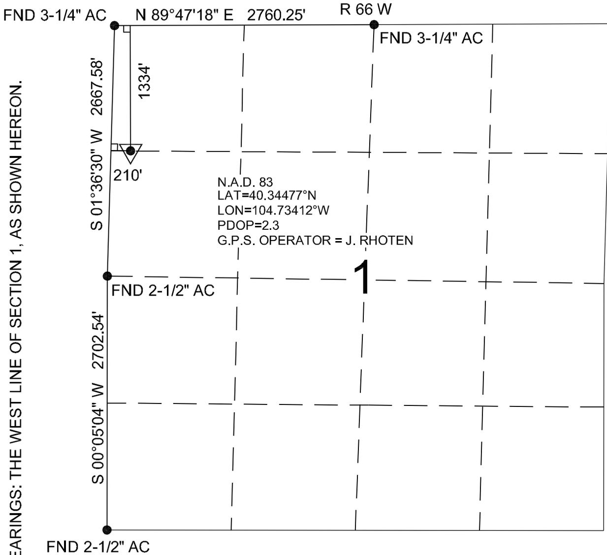
BASIS OF BEARINGS: THE WEST LINE OF SECTION 1, AS SHOWN HEREON.
