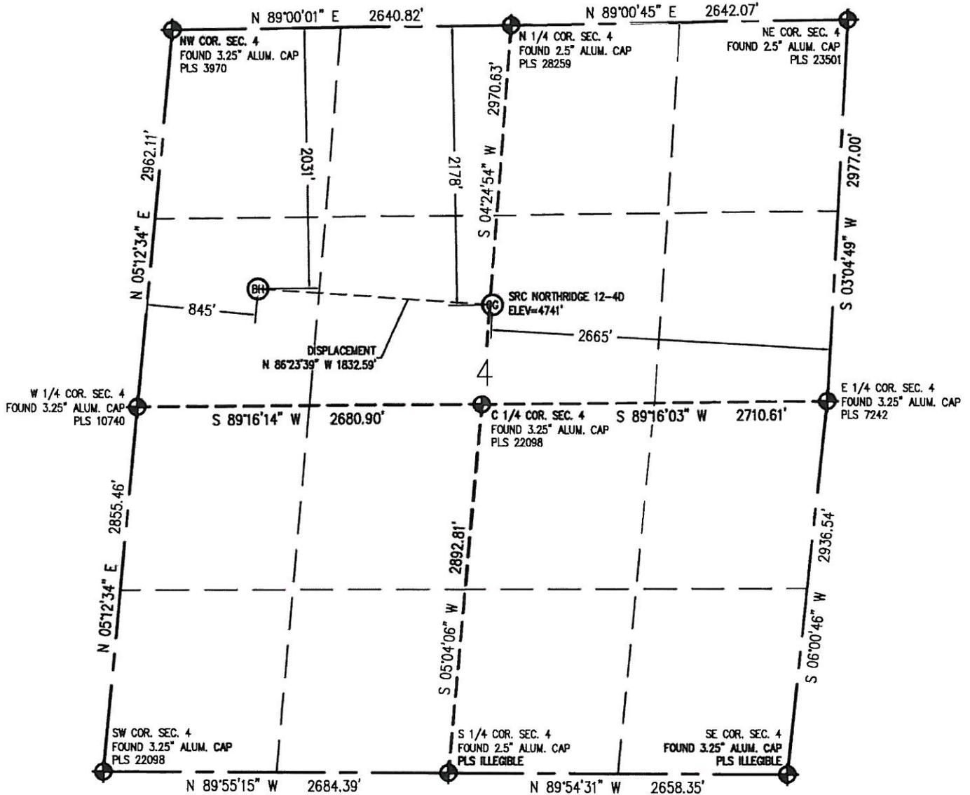
IN ACCORDANCE WITH A REQUEST FROM CRAIG RASMUSON - SYNERGY RESOURCES, BASELINE ENGINEERING CORP. HAS DETERMINED THE LOCATION OF THE SRC NORTHBRIDGE 12-40 TO BE 2178' FNL AND 2665' FEL, AS MEASURED AT NINETY (90) DEGREES FROM THE SECTION LINE OF SECTION 4, TOWNSHIP 5 NORTH, RANGE 66 WEST AND THE BOTTOM HOLE LOCATION TO BE 2031' FNL AND 845' FNL OF SECTION 4, TOWNSHIP 5 NORTH, RANGE 66 WEST, 6TH PRINCIPAL MERIDIAN, WELD COUNTY, COLORADO.
