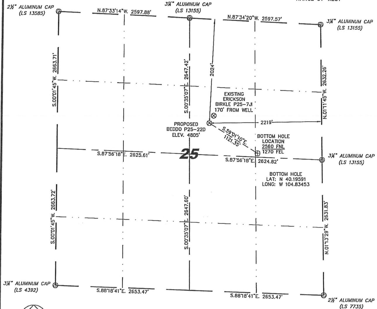
IN ACCORDANCE WITH A REQUEST FROM MATT CAMPBELL - NOBLE ENERGY INC, STELL SURVEYING SERVICES, LLC HAS DETERMINED THE LOCATION OF THE BEDDO P25-22D WELL TO BE 2024' FNL, 2219' FEL, AS MEASURED AT NINETY (90) DEGREES FROM THE SECTION LINES, SECTION 25, TOWNSHIP 3 NORTH, RANGE 67 WEST, 6TH PRINCIPLE MERIDIAN, WELD COUNTY, COLORADO.
