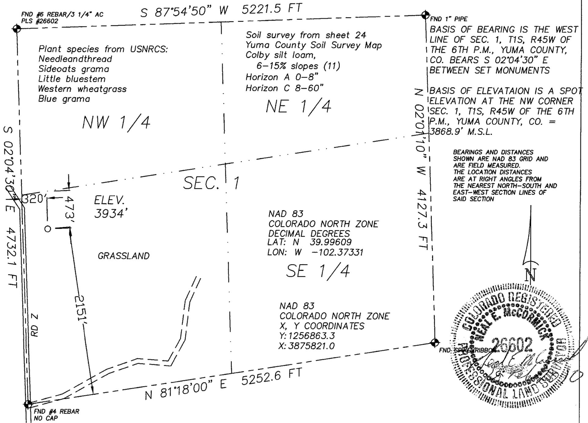
BEARINGS AND DISTANCES SHOWN ARE NAD 83 GRID AND ARE FIELD MEASURED. THE LOCATION DISTANCES ARE AT RIGHT ANGLES FROM THE NEAREST NORTH-SOUTH AND EAST-WEST SECTION LINES OF SAID SECTION
