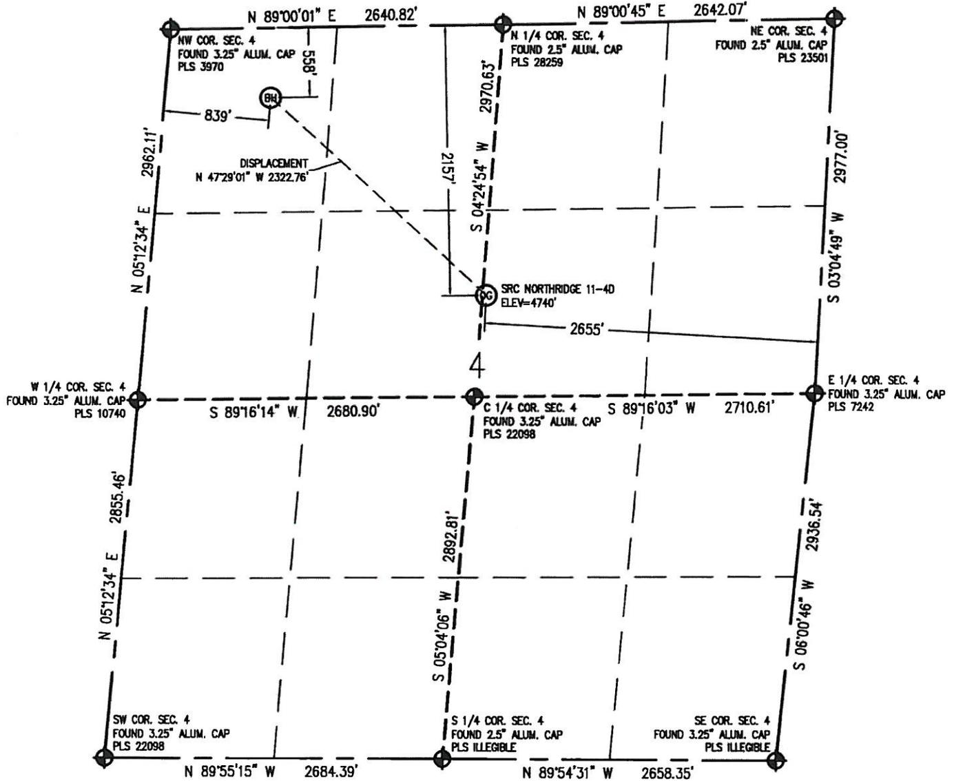
IN ACCORDANCE WITH A REQUEST FROM CRAIG RASMUSON - SYNERGY RESOURCES, BASELINE ENGINEERING CORP. HAS DETERMINED THE LOCATION OF THE SRC NORTHRIDGE 11-4D TO BE 2157' FNL AND 2655' FEL, AS MEASURED AT NINETY (90) DEGREES FROM THE SECTION LINE OF SECTION 4, TOWNSHIP 5 NORTH, RANGE 66 WEST AND THE BOTTOM HOLE LOCATION TO BE 558' FNL AND 839' FWL OF SECTION 4, TOWNSHIP 5 NORTH, RANGE 66 WEST, 6TH PRINCIPAL MERIDIAN, WELD COUNTY, COLORADO.
